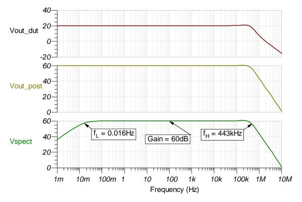
Figure 9: Bandwidth of Noise Post Amplifier
