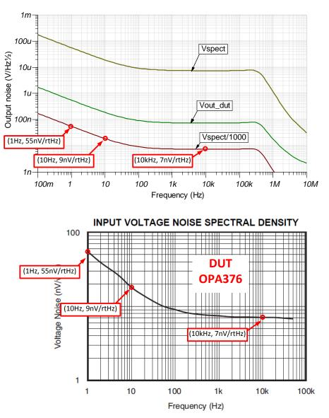
Figure 7: Simulated Noise Spectral Density vs. Specified
