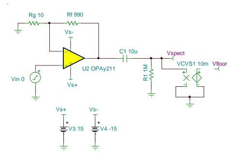
Figure 11: Post Amp Noise Floor Simulation
