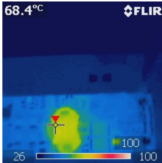
Vin=40V Iout=0A, Hot spot is Transformer core. 0 cfm
