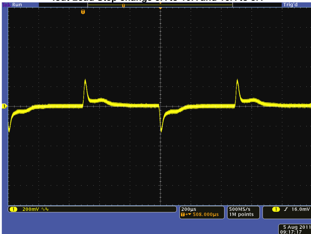
Vout response with 50% step change in load. External capacitance=150uf
