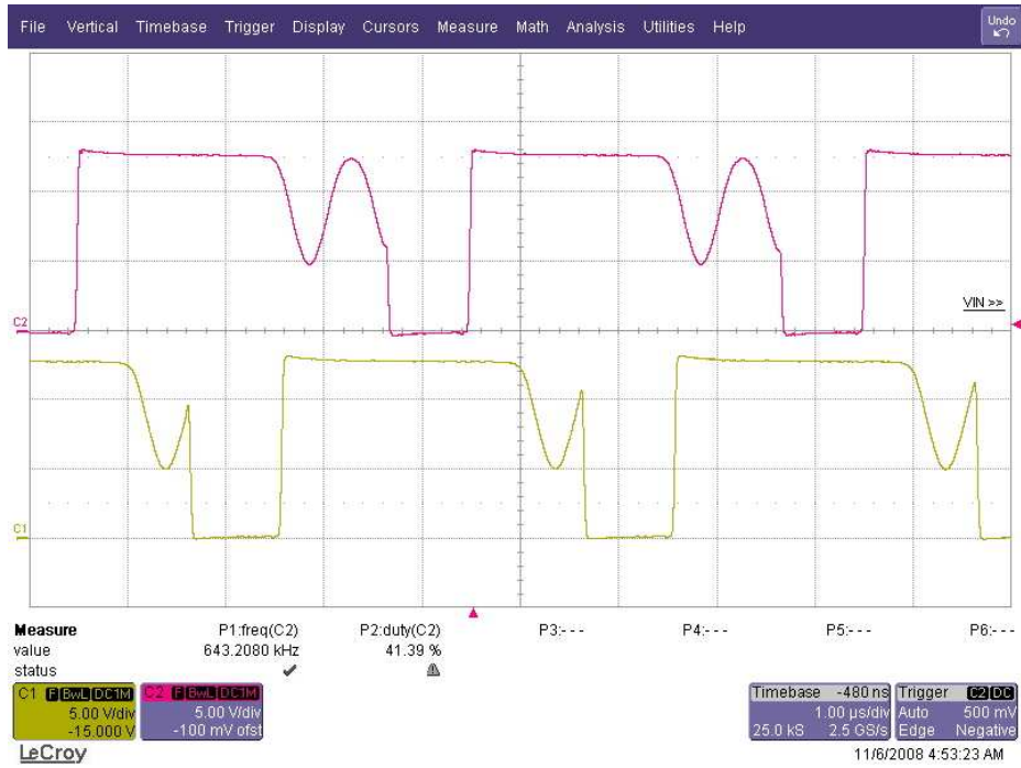
Current Sharing 1 (Iout<0.5A Vin=9V): VdsQ1, VdsQ2
