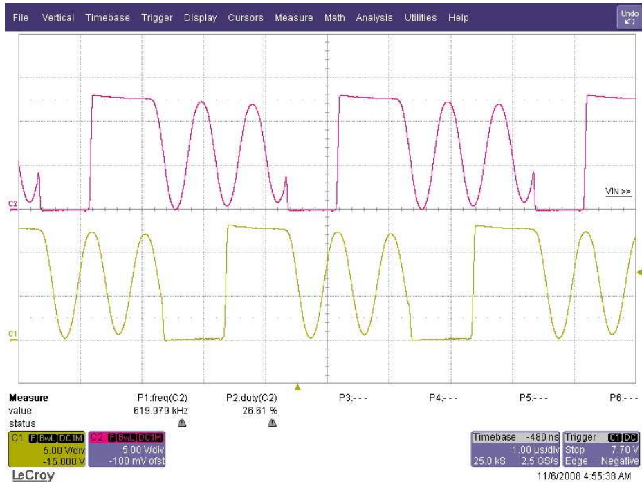
Current Sharing 2 (Iout<0.15A Vin=6.5V): VdsQ1 (C1), VdsQ2 (C2)
