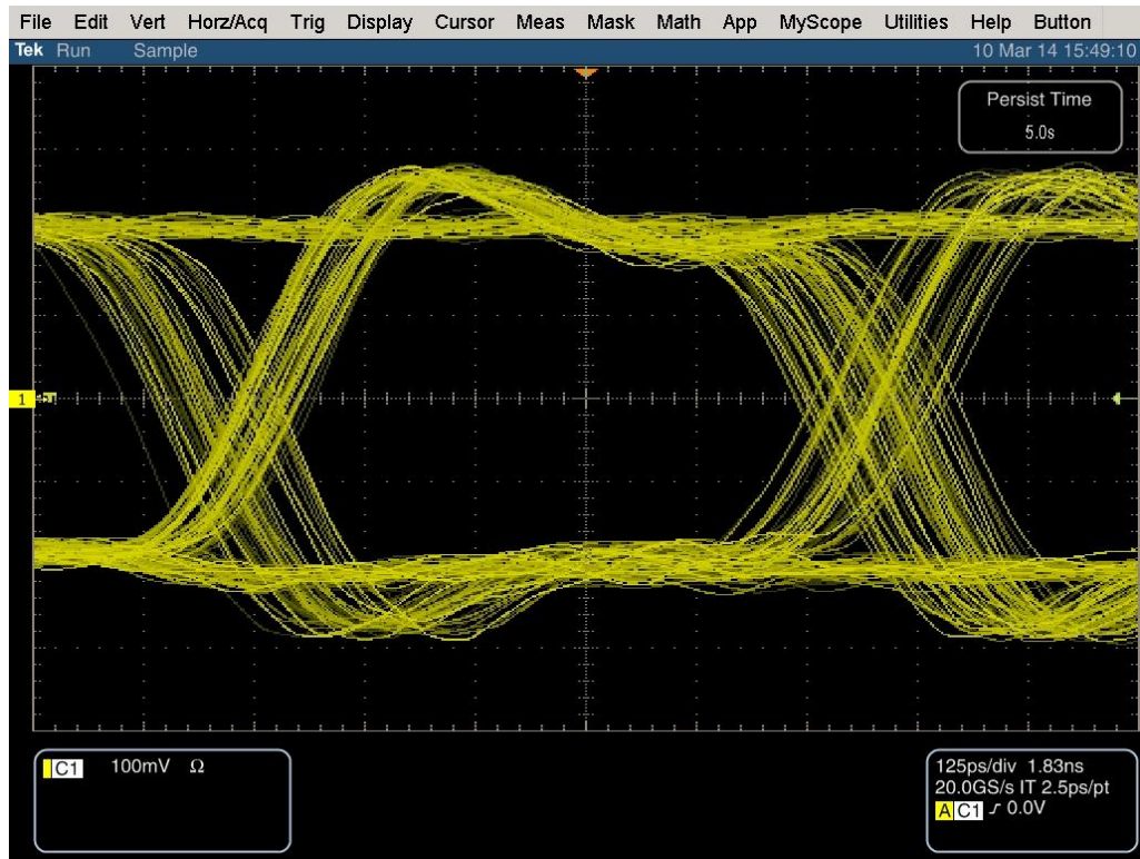
Figure 1: Eye diagram of DS90UB914A-CXEVM and DS90UB913A-CXEVM
