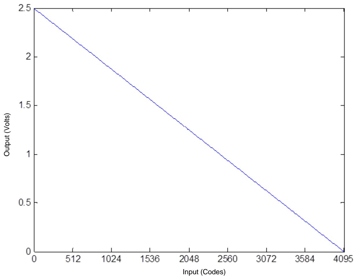
**Figure 1: Measured Transfer Function**
