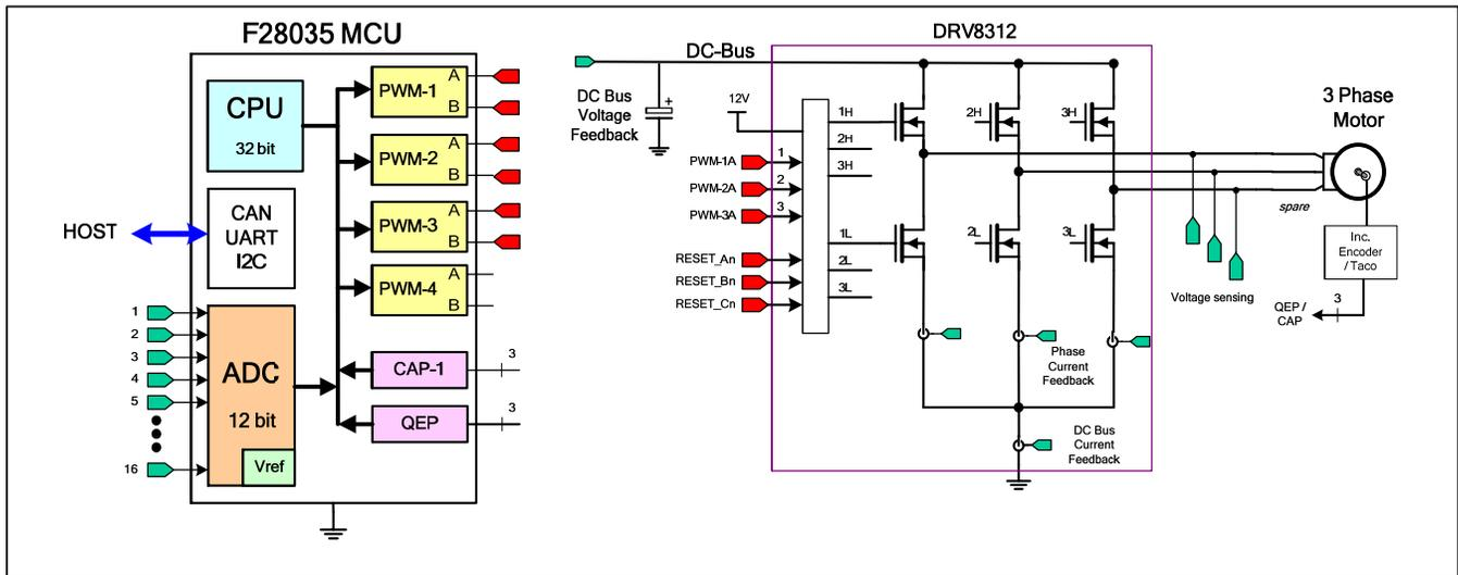
Figure 7. Medium Voltage DMC Board Block Diagram with C2000 MCU
