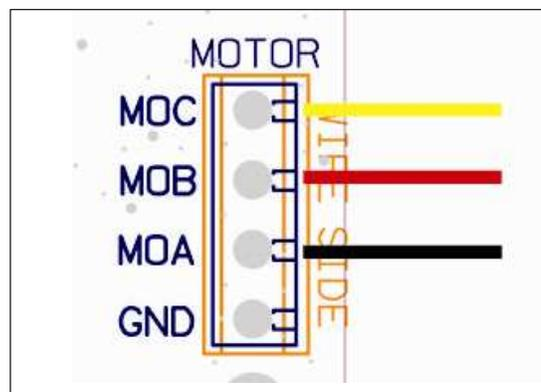
**Figure 6. DRV8312-EVM Motor Connections**
