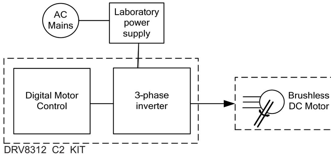
Figure 4. Block Diagram for a Typical Motor Drive System
