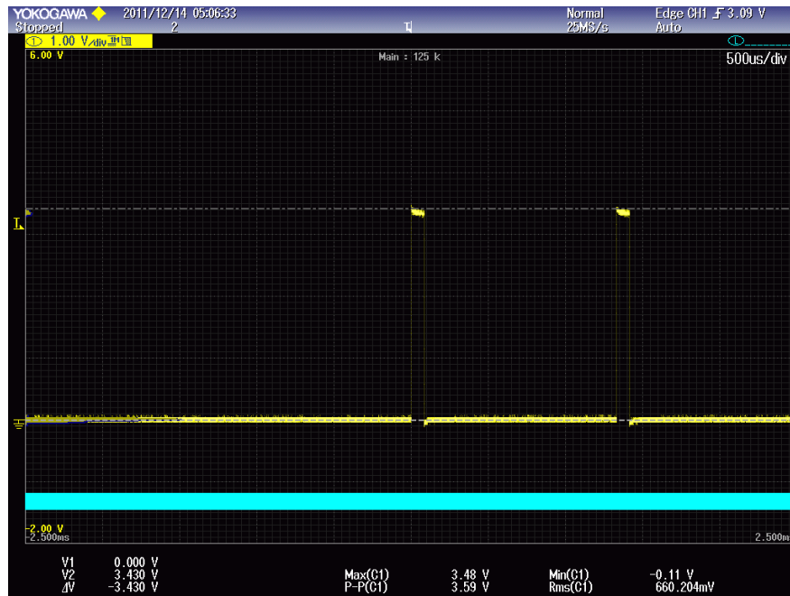
Figure 2 - HEART signal, bottom module to oscilloscope (or microcontroller)
