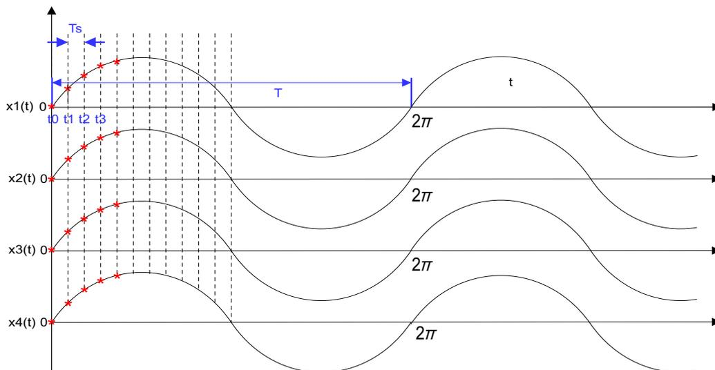
**Figure 6. Simultaneous Sampling for Four Channel Signals**
