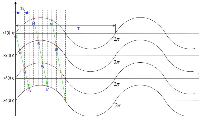
**Figure 7. Non-Simultaneous Sampling for Four Channel Signals**
