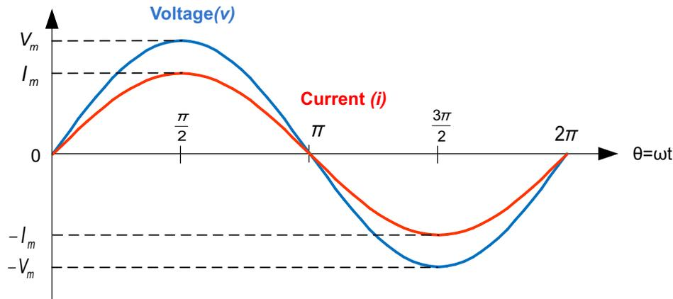
**Figure 3. Two Sinusoidal Waveforms—“In-Phase”**
