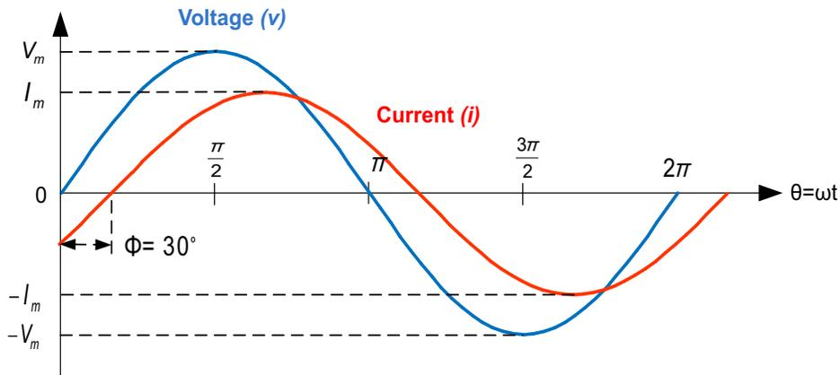
**Figure 4. Phase Difference of Two Sinusoidal Waveforms**
