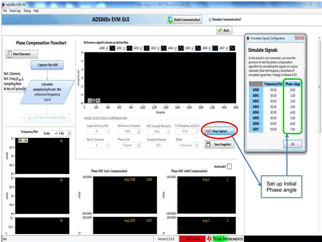
Figure 17. Phase Compensation With Initial Phase Angle Setup
