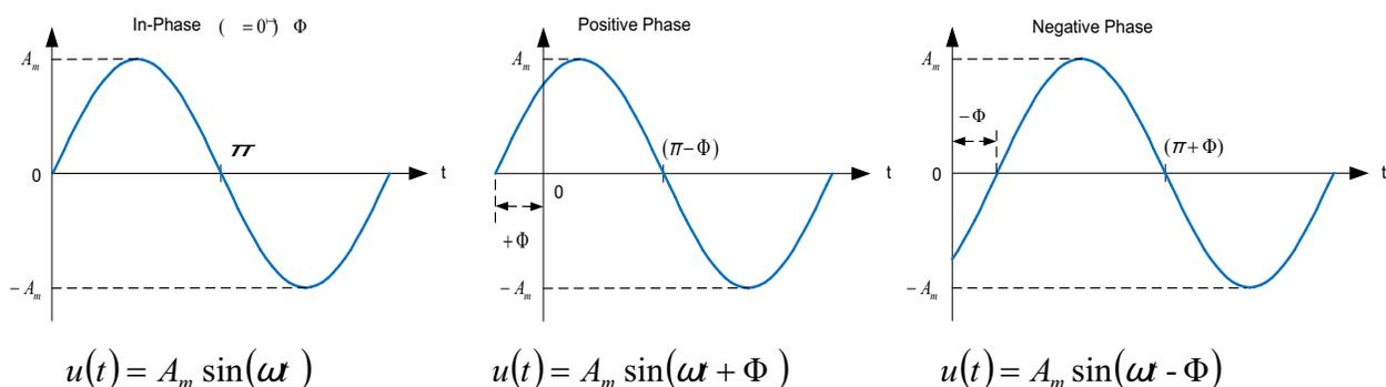
**Figure 2. Illustration of Positive, Negative, and Zero Phase for Sinusoidal Signal**
