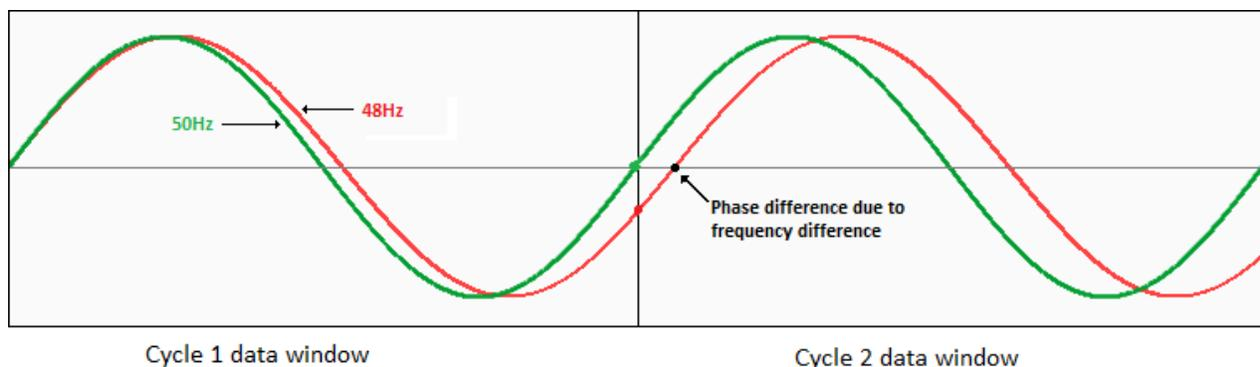
**Figure 8. Phase Difference as Result of Frequency**
