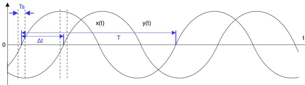
**Figure 21. Calculation Chart of Phase Difference for First-order Linear Interpolation**
