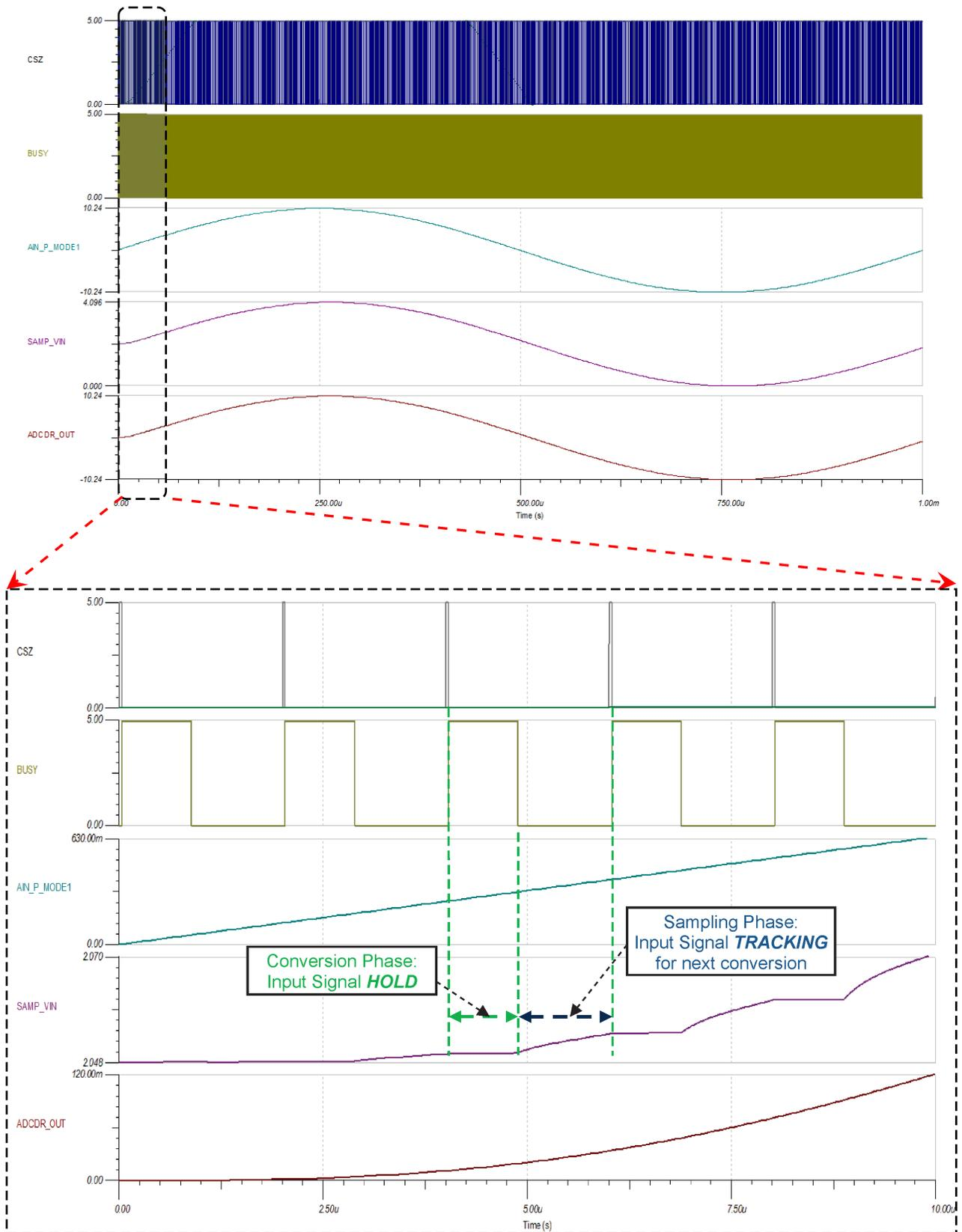
Figure 12. TINA-TI™ Model Simulation for Sinusoidal Waveform Input—MODE1
