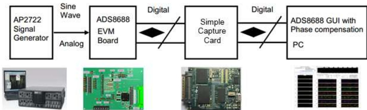
Figure 14. Test Connection and Flow Chart
