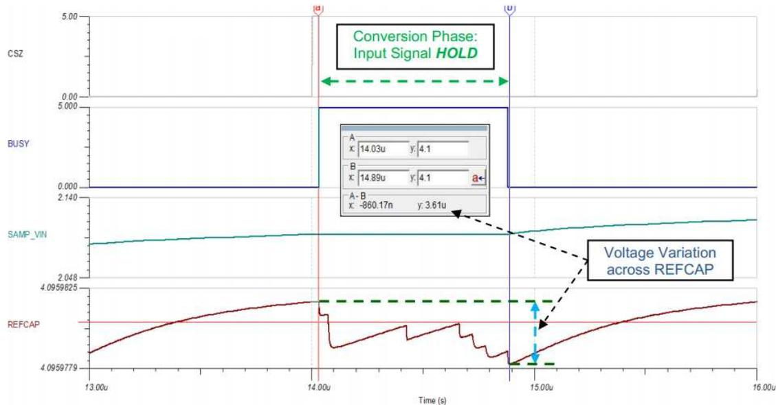
**Figure 13. Voltage Change Across Reference Capacitor During Conversion Time**
