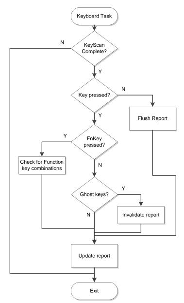
Figure 13. Flow Diagram for Keyboard Task
