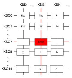
Figure 8. Detection of a Key Using Polling Method
