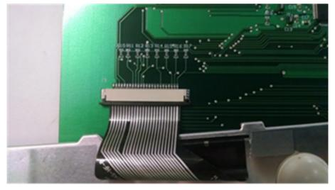
Figure 18. Keyboard Connection
