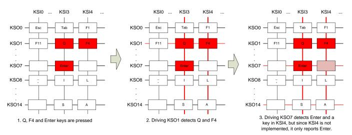
Figure 10. Ignored "Ghost" Key Condition Due to Unimplemented Key
