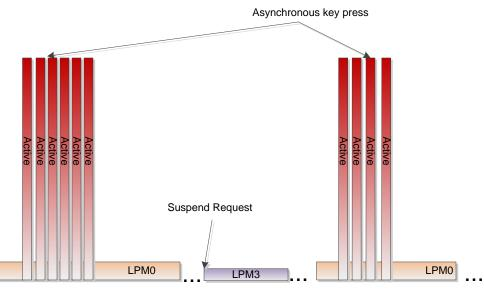
Figure 29. Expected Power Profile for USBKBD Configuration
