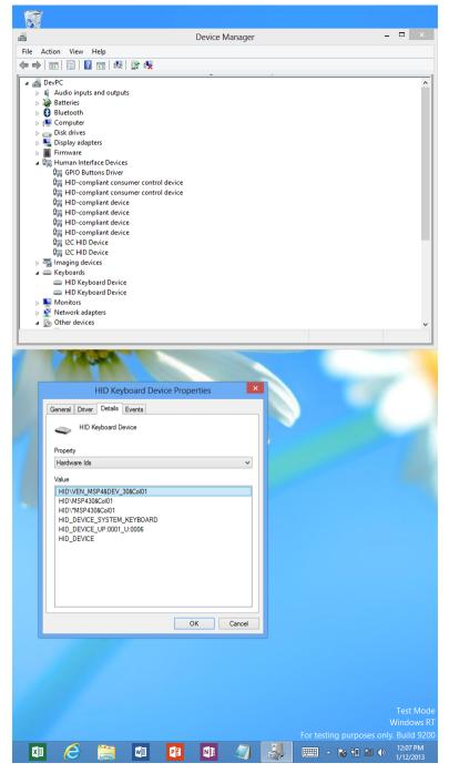
Figure 21. I2C Keyboard in Windows Device Manager
