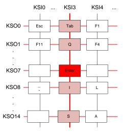
Figure 7. Detection of a Key Using Column-Interrupt Method
