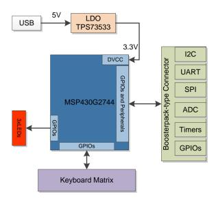
Figure 4. Block Diagram using MSP430G2744
