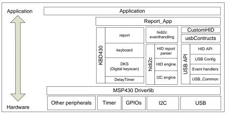
Figure 11. Software Architecture
