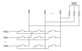
Figure 6. Keyboard Schematic Model
