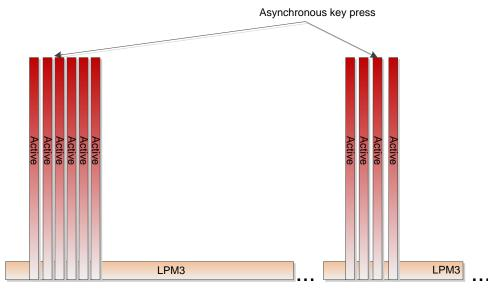
Figure 27. Expected Power Profile for I2CKBD and I2CKBD\_G2xx4 Configurations
