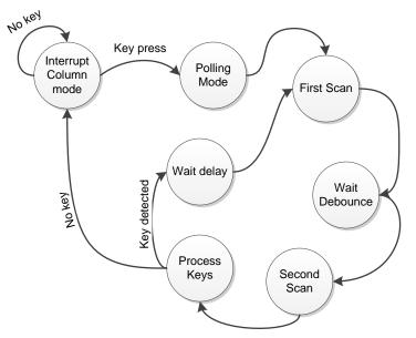
Figure 14. State Diagram for Keyboard Scan
