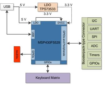
Figure 3. Block Diagram using MSP430F5529
