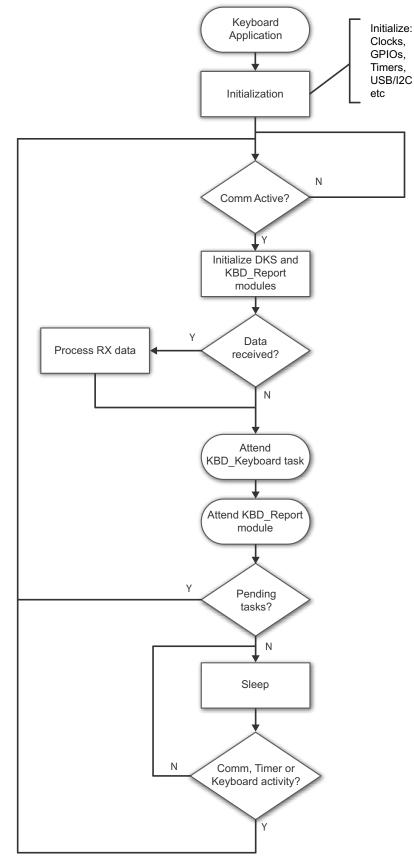
Figure 12. Application Flow Diagram
