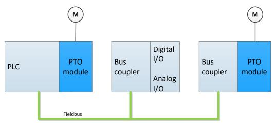
Figure 1. PLC Application With PTO Modules
