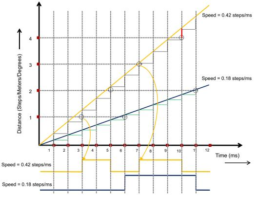
Figure 11. Two Speed Examples With the Generation of PTO Output
