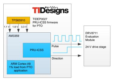
Figure 9. PTO Block Diagram
