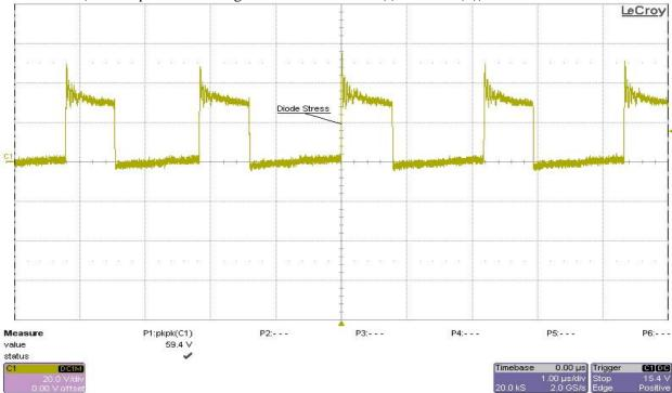
$Ch1-Vd12\ (12V\ output\ diode\ voltage\ stress\ from\ cathode\ (-)\ to\ anode\ (+))$
