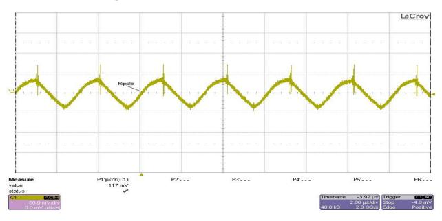
Test condition: The input voltage was set at 24V, and all outputs were set at full load. Ch1 - 5VP (+5V) (AC coupled)
