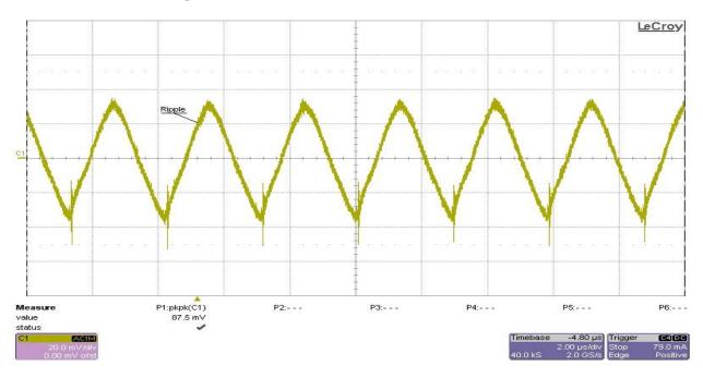
Test condition: The input voltage was set at 24V, and all outputs were set at full load. Ch1 - 5VP (+5V) (AC coupled)
