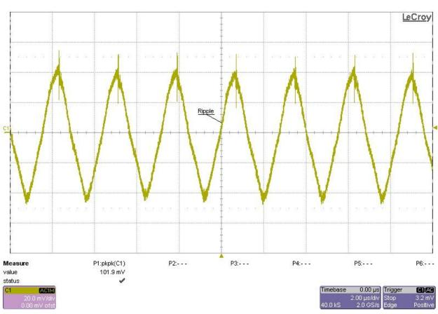
Test condition: The input voltage was set at 24V, and all outputs were set at full load. Ch1 - 12VN (-12V) (AC coupled)
