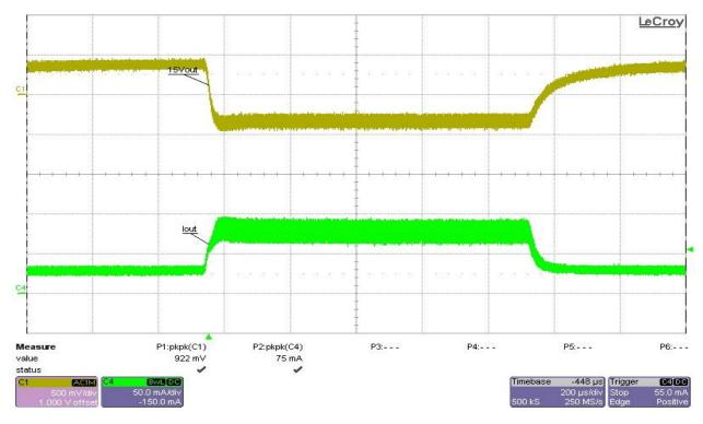
Test condition: Vin = 24V, 15VP (+15V) load from 0A to 50mA, no load at the other outputs. Ch1- 15VP (+15V) (AC mode), Ch4- Io (+15V output current)
