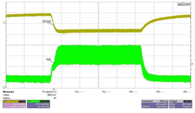
Test condition: Vin = 24V, 24VP (+24V) load from 0A to 25mA, no load at the other outputs. Ch1- 24VP (+24V) (AC mode), Ch4- Io (+24V output current)
