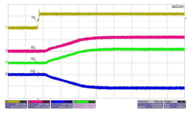
Test condition: The input voltage was set at 30V, and all outputs were set at full load. Ch1 - Vin, Ch2 - 12VP(+12V), Ch3 - 5VP(+5V), Ch4 - 12VN(-12V)
