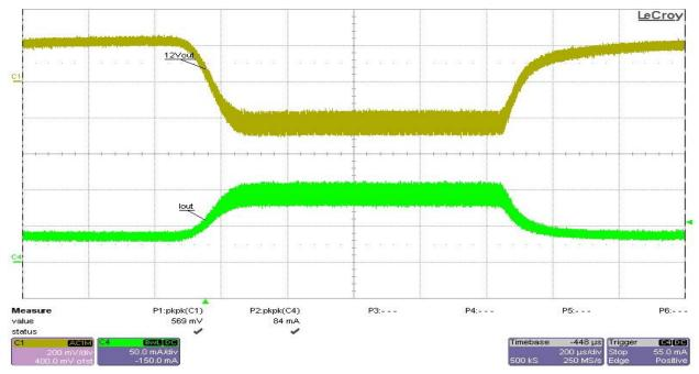
Test condition: Vin = 24V, 5VP (+5V) load from 0A to 100mA, no load at the other outputs. Ch1- 5VP (+5V) (AC mode), Ch4- Io (+5V output current)
