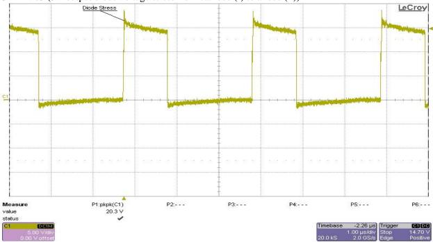
Ch1 - Vd5 (5V output diode voltage stress from cathode (-) to anode (+))
