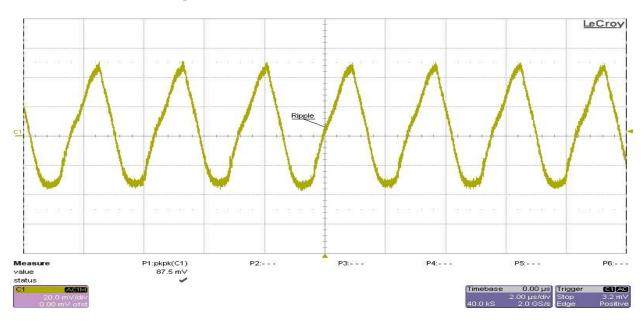
Test condition: The input voltage was set at 24V, and all outputs were set at full load. Ch1 - 24VP (+24V) (AC coupled)
