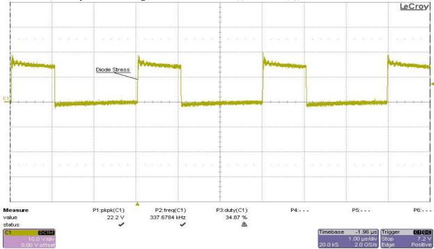
Ch1 - Vd5 (5V output diode voltage stress from cathode (-) to anode (+))
