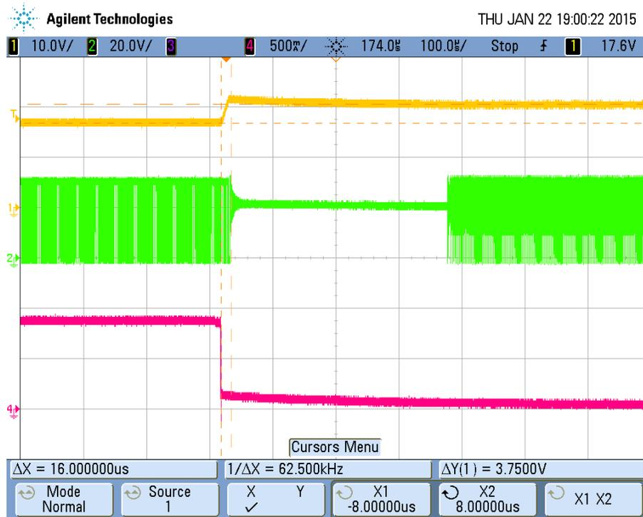
Figure 13 Open circuit test from 700mA output operation
