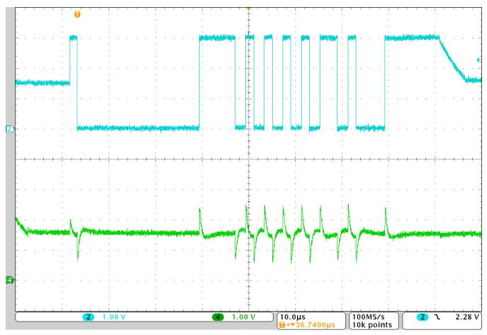
Figure 11. ABR Detection — Break/Synch Sequence Plus One Data Byte
