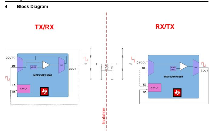
Figure 2. TIDA-00245 Block Diagram
