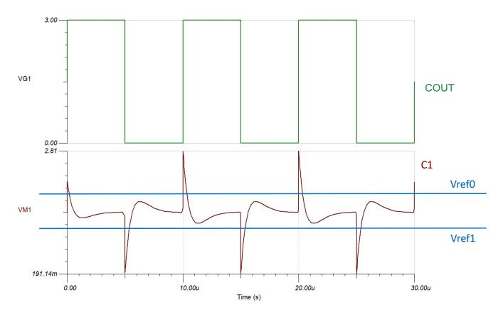
Figure 5. Comparator Input and Output Signal
