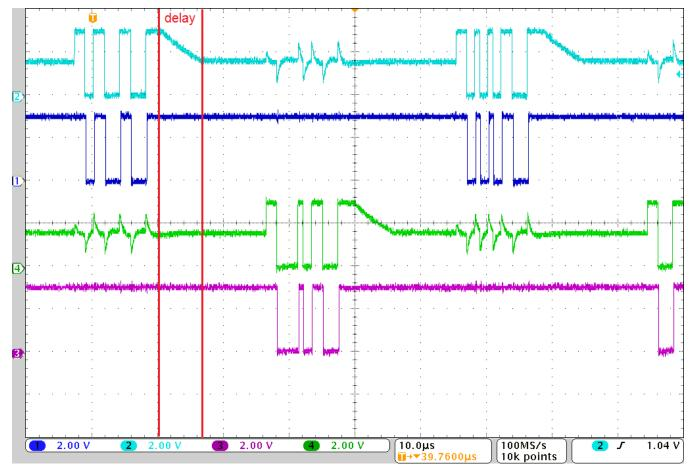
Figure 8. Bidirectional Data Communication
