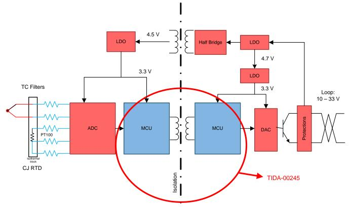
Figure 1. Isolated Thermocouple Sensor
