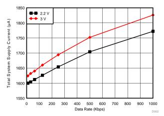
Figure 14. Total Supply Current in Bidirectional Mode
