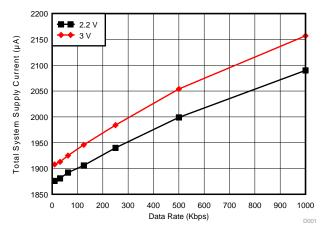
Figure 13. Total Supply Current in Unidirectional Mode
