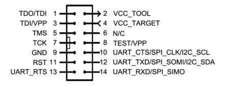
Figure 9: MSP- FET JTAG Connector Pinout
