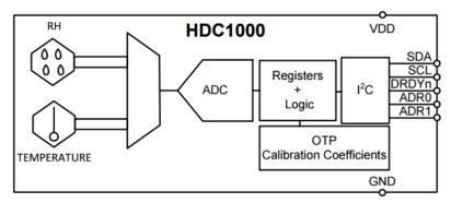
Figure 5: HDC1000 Block Diagram
