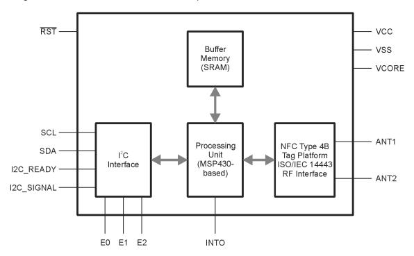
Figure 2: RF430CL331H Block Diagram
