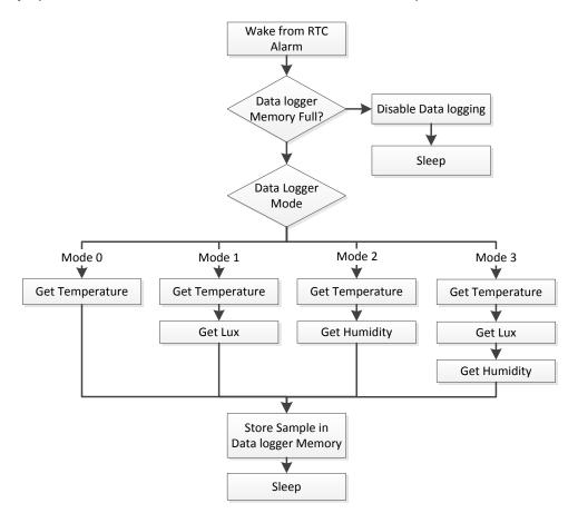
Figure 13: Data Logger State Diagram
