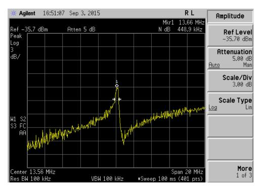
Figure 17: Resonant Frequency
