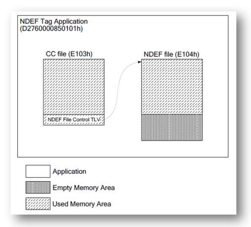
Figure 14: NDEF tag Application Mapping Example
