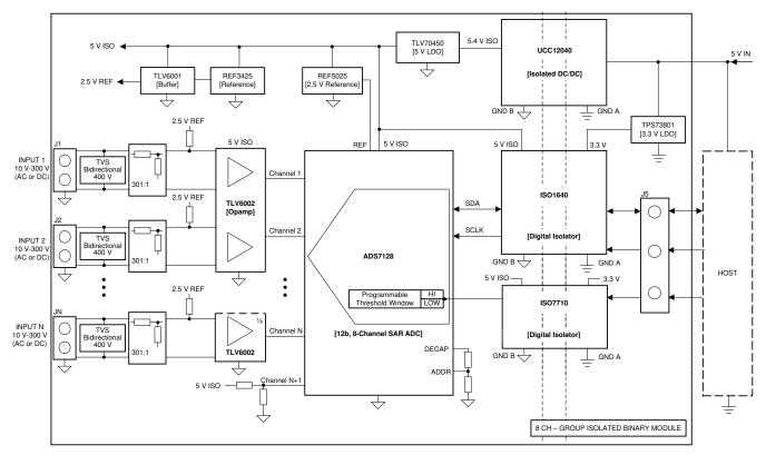
Figure 2-2. Block Diagram of ADC-based BIM Design (ADS7128)
