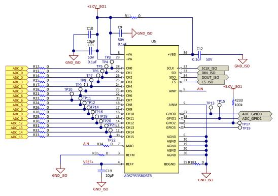
Figure 3-1. ADC Configuration for Measuring Multiple Channels
