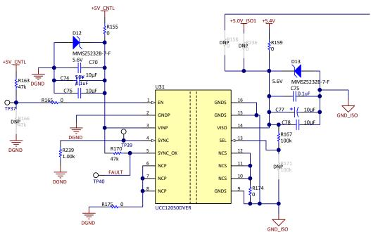
Figure 3-4. Reinforced Isolation DC/DC Converter Power Supply
