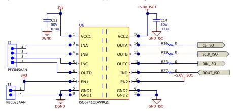
Figure 3-3. Reinforced Digital Isolator for Host Interface (SPI)
