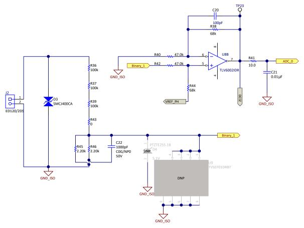
Figure 3-2. Signal Conditioning Operational Amplifier and Voltage Divider
