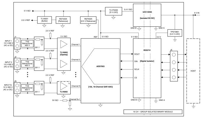
Figure 2-1. Block Diagram of ADC-based Binary Input Module
