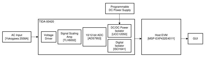
Figure 4-1. Test Setup Layout
