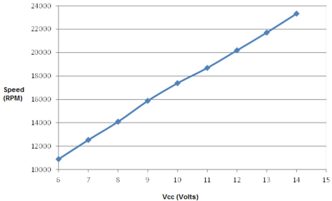
Figure4: Motor Speed with respect to Vcc
