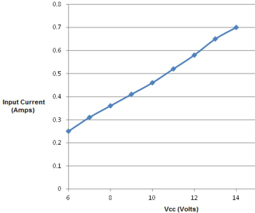
Figure 2: Input Current with respect to Vcc
