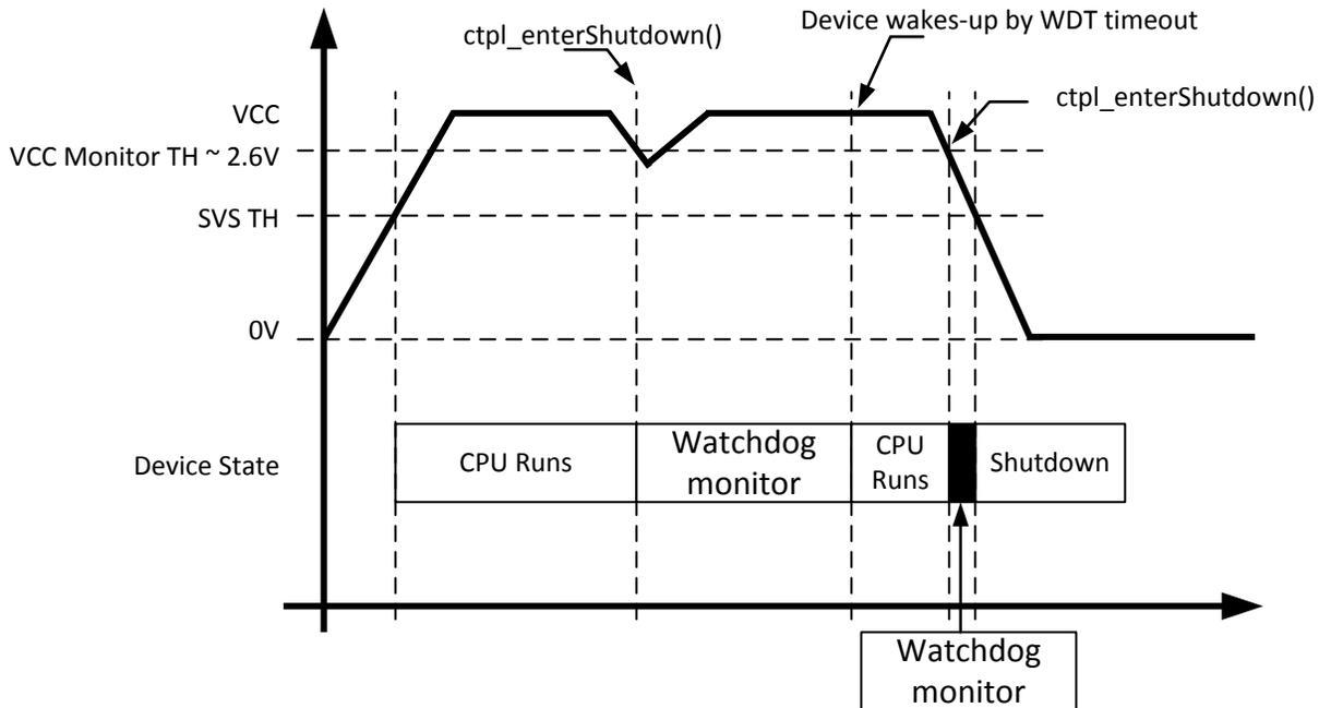
**Figure 5. Power-Up and Down Conditions**
