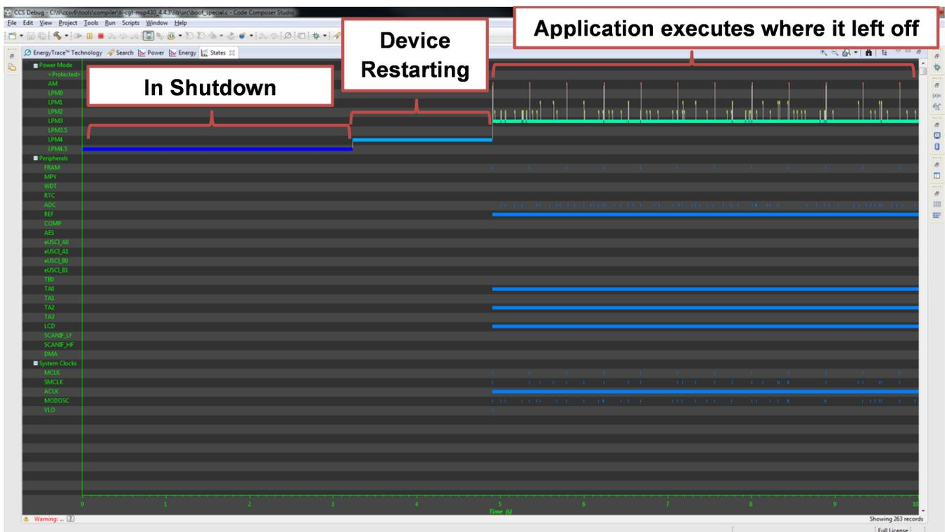
Figure 9. EnergyTrace++ Capture of Application Waking Up From CTPL Shutdown
