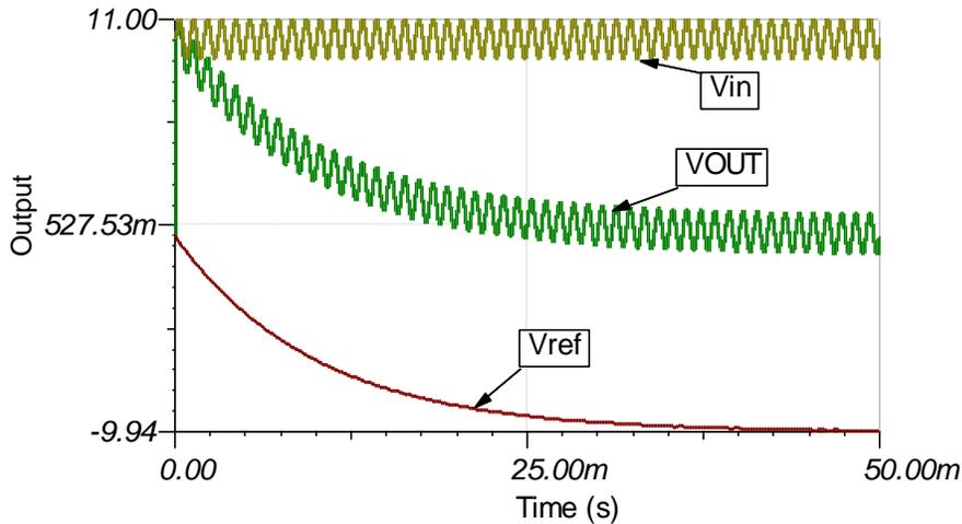
**Figure 5: Startup Transient Integrator Ramping to Cancel Output Offset**
