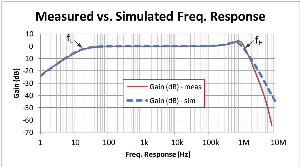
Figure 4: Frequency response for INA118 and OPA188 dc rejection circuit
