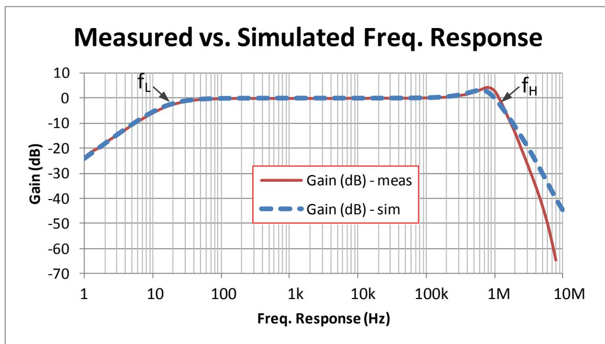
Figure 3: Lower and upper cutoff frequency shown on ac transfer characteristic
