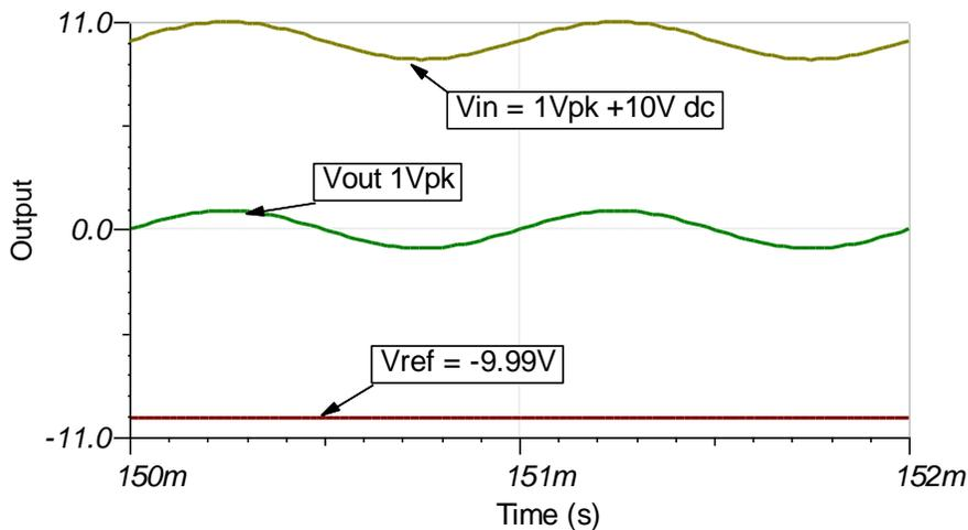
**Figure 6: Steady State Transient to 1Vpk+10Vdc 1kHz Input Signal**
