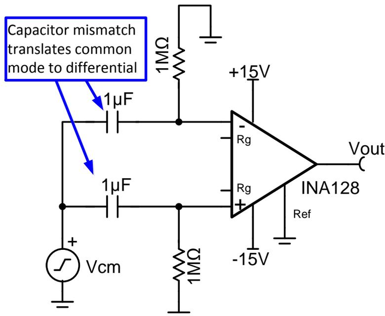
Figure 9: ac Coupled with Input Capacitors Error Source - Common Mode to Differential Translation
