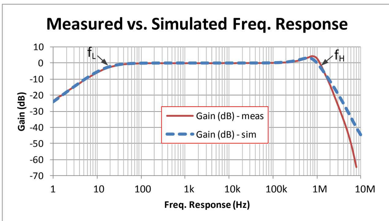
**Figure 1: Simulated and Measured Transfer Function**
