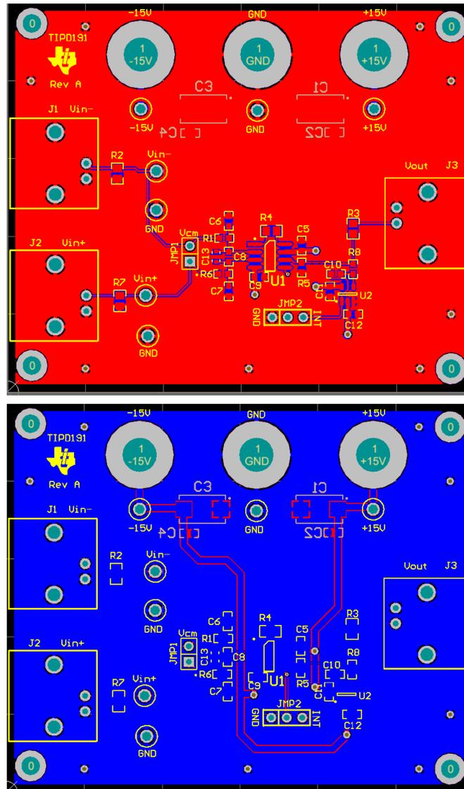
Figure 7: PCB Layout (Top - Red, Bottom - Blue)
