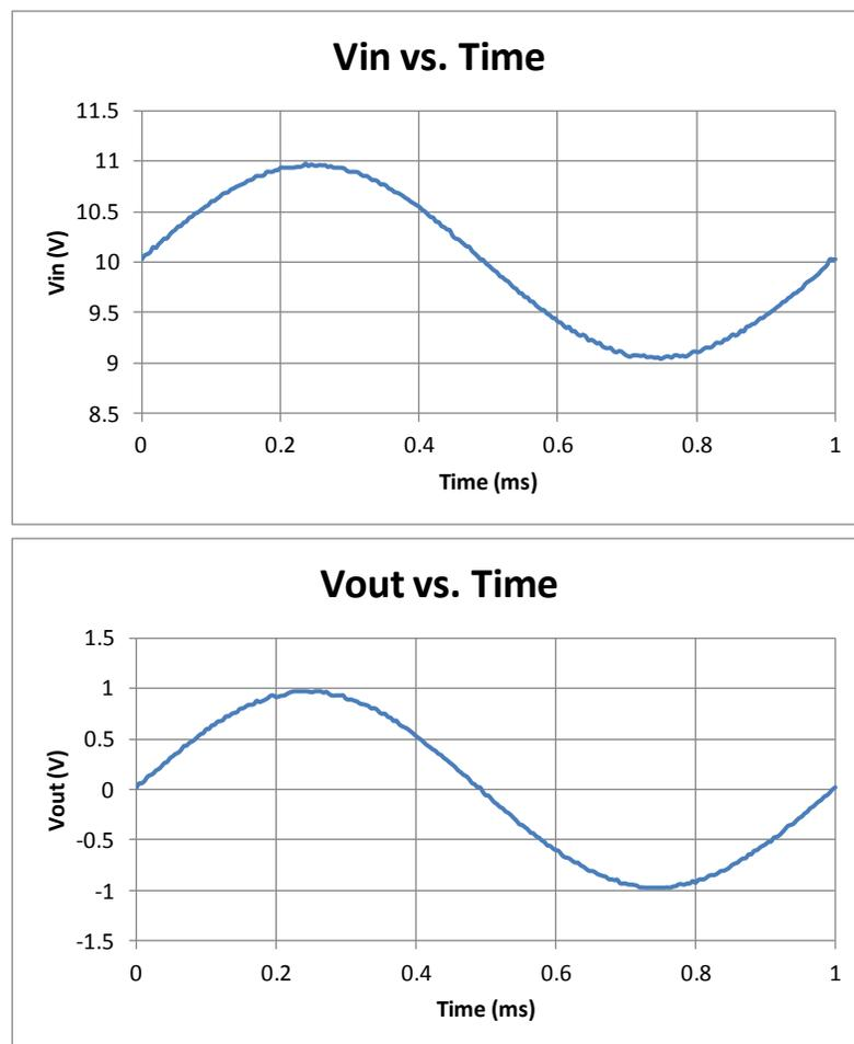
**Figure 8: Transient Response to a 1Vpk 1kHz + 10Vdc Input Signal**
