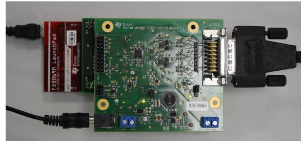
Figure 31. TIDA-00176 Board Mounted on InstaSPIN-MOTION LaunchPad
