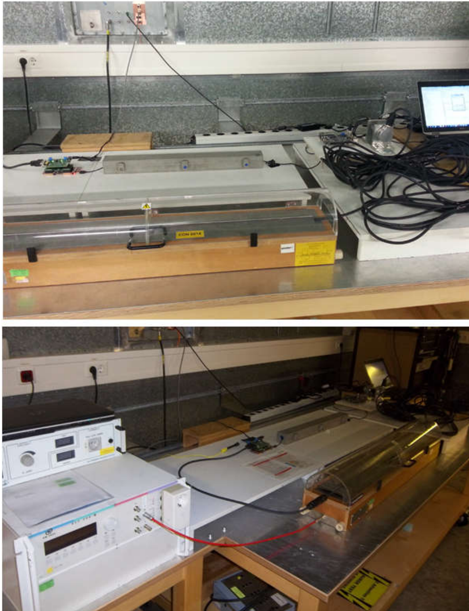
Figure 7-39. IEC61000-4-4 EFT Test Setup for TIDA-00176 (Right Side on Top, Left Side on Bottom)
