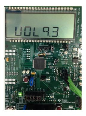
Figure 9. Volume Displayed on LCD
