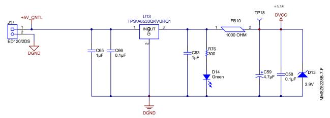
Figure 12. Non-Isolated Power Supply With Zener Protection
