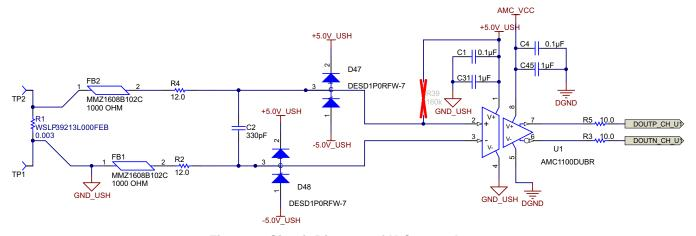
Figure 9. Circuit Diagram of U Current Input
