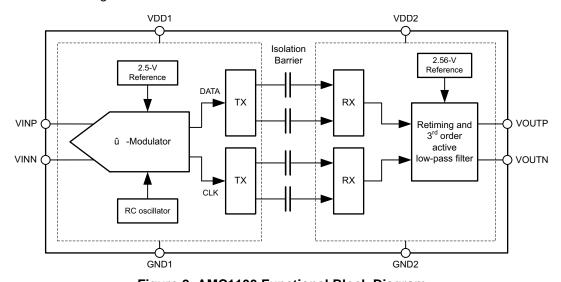
Figure 2. AMC1100 Functional Block Diagram
