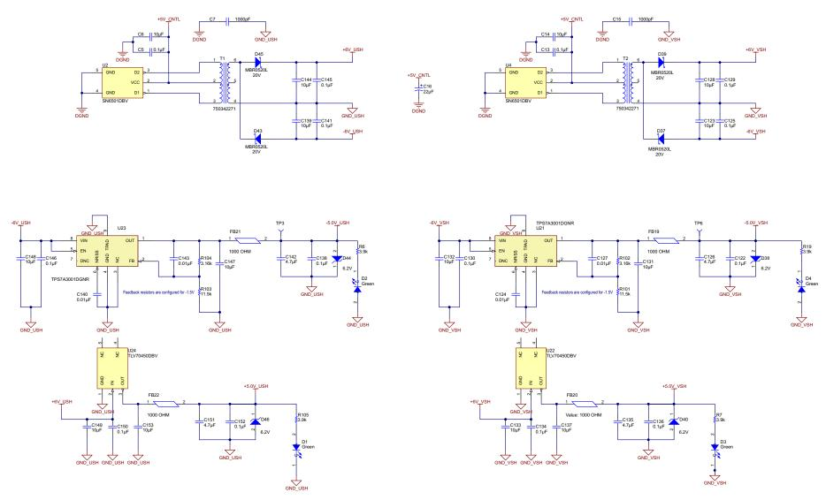
Figure 37. TIDA-00555 Schematic—Regulators
