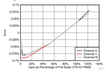
Figure 27. Voltage Measurement Error for U, V, and W Channels
