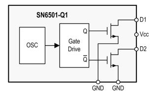
Figure 3. SN6501 Functional Block Diagram
