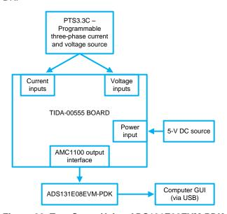
Figure 22. Test Setup Using ADS131E08EVM-PDK
