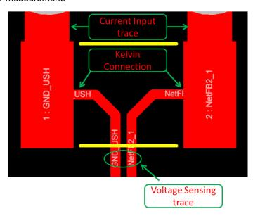
Figure 39. TIDA-00555 Shunt Layout
