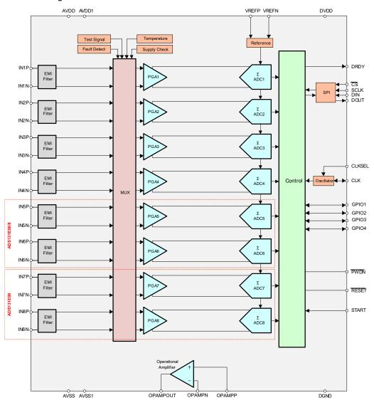
Figure 7. ADS131E08 Functional Block Diagram
