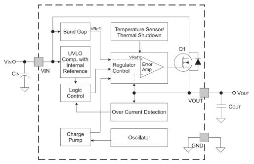
Figure 6. TPS7A6533 Functional Block Diagram
