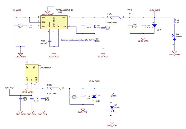
Figure 11. Isolated Power Supply and Zener Protection Schematics
