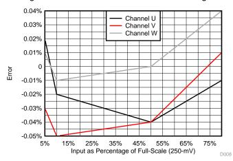
Figure 31. Voltage Measurement Error for U, V, and W Channels
