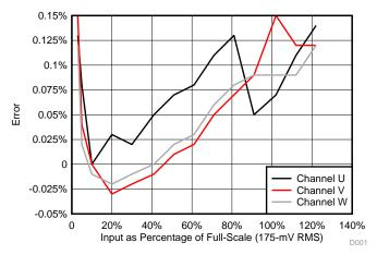
Figure 24. Voltage Measurement Error for U, V, and W Channels
