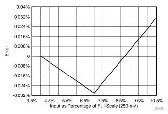
Figure 32. Current Measurement Error for U Channel
