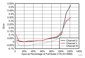
Figure 26. Voltage Measurement Error for U, V, and W Channels
