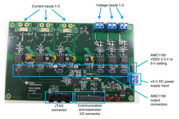
Figure 18. TIDA-00555 Interface Connectors
