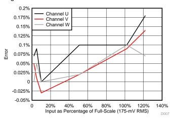
Figure 30. Voltage Measurement Error for U, V, and W Channels
