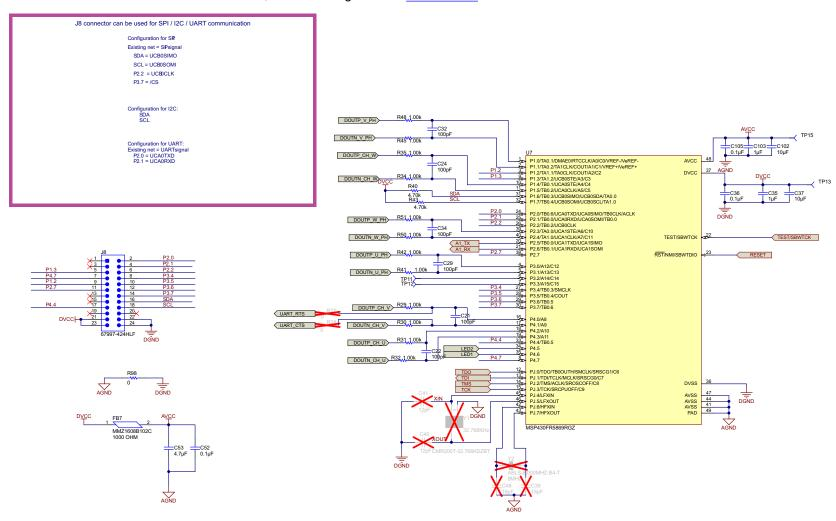
Figure 33. TIDA-00555 Schematic—MCU
