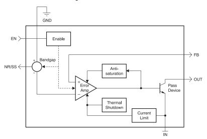
Figure 5. TPS7A30 Functional Block Diagram
