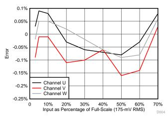
Figure 28. Current Measurement Error for U, V, and W Channels
