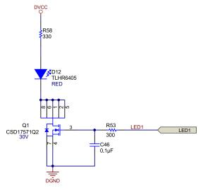
Figure 16. LED Schematic
