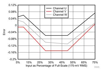
Figure 29. Current Measurement Error for U, V, and W Channels
