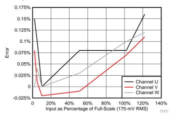
Figure 25. Voltage Measurement Error for U, V, and W Channels
