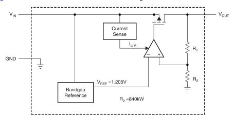
Figure 4. TLV704 Functional Block Diagram
