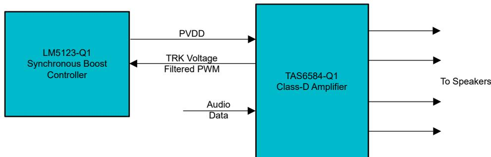
**Figure 1-1. Simplified Class-H System With TAS6584-Q1 and LM5123-Q1**
