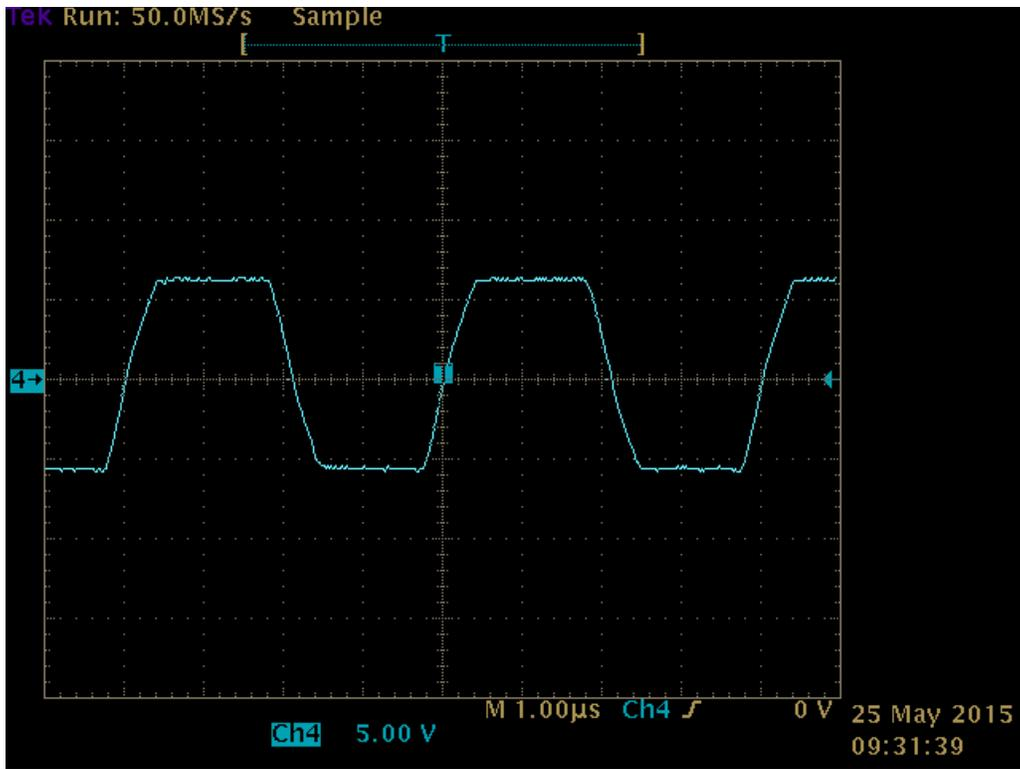
Figure 2. RS-232 transmitting signal (500 kbps)
