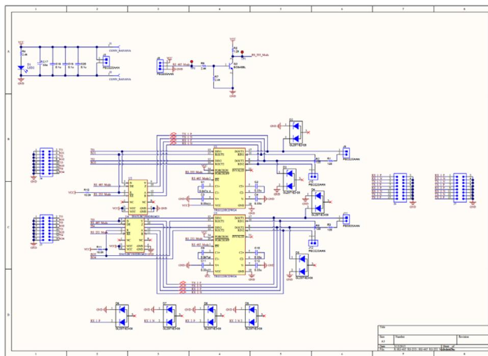
**Figure 1. RS232/RS485 multiprotocol transceivers schematic**
