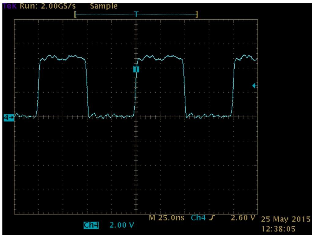
Figure 5. RS-485 receiving single-ended signal (20 Mbps)
