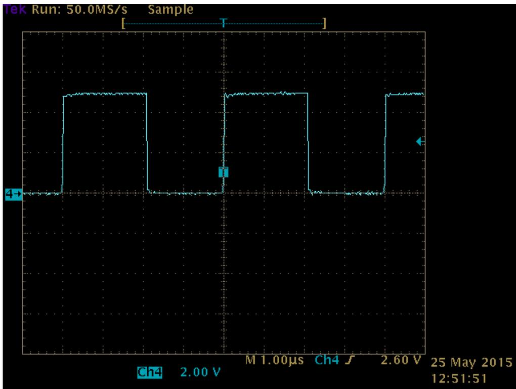
Figure 3. RS-232 receiving single-ended signal (500 kbps)
