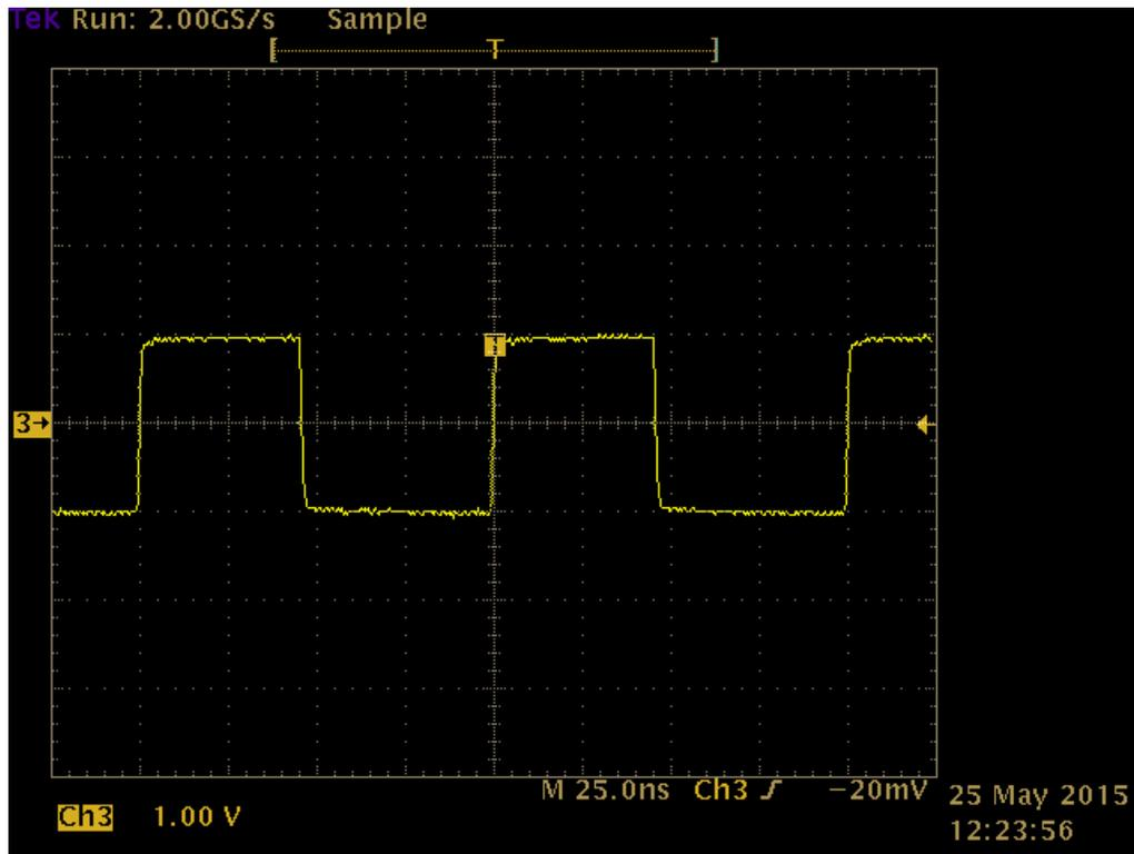
Figure 4. RS-485 transmitting differential signal (20 Mbps)
