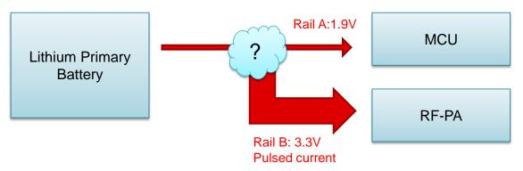
Figure 1: Smart Wireless Sensor Node - Power Block-Diagram
