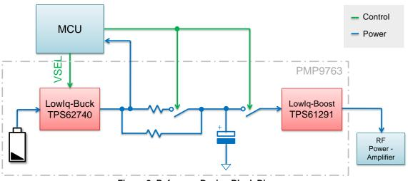
Figure 2: Reference Design Block Diagram
