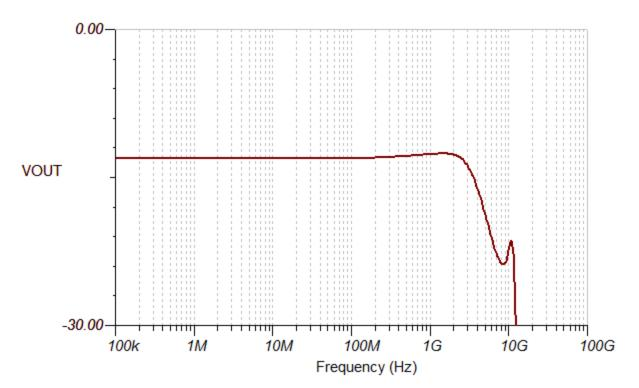
Figure 11 Simulation Results for Av =0.5 V/V, Approximating Measured Results (see schematic in Figure 10)
