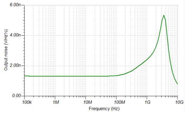
Figure 6 TINA-TI Noise Simulation, Av =0.5, Rs=255 Ohms, Noise Gain = 3
