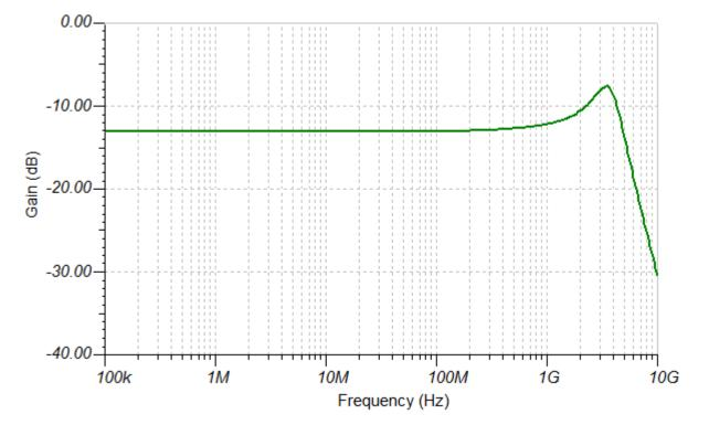
Figure 4 Gain = 0.5 V/V Frequency response, noise gain = 3V/V
