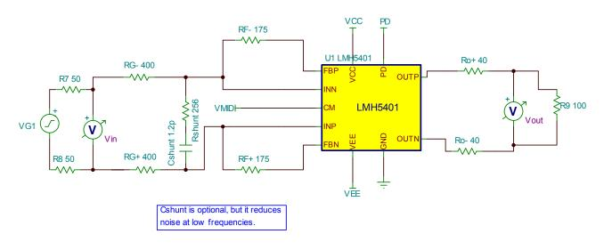
Figure 5 Gain = 0.5V/V, Noise Gain = 3V/V
