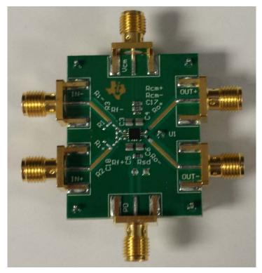
Figure 1 Reference Design Board
