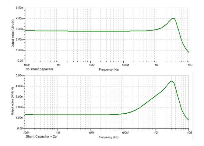
Figure 8 TINA-TI Noise Simulation, Av =0.5, Rs=154 Ohms, noise gain = 4 (Top plot no Cshunt, Bottom plot, Cshunt = 2p)
