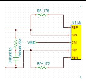
Figure 3 Stabilizing shunt resistor shown as Rshunt
