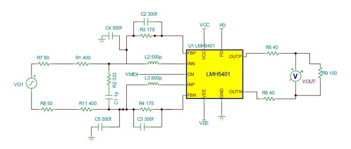
Figure 10 Adjusted TINA Schematic
