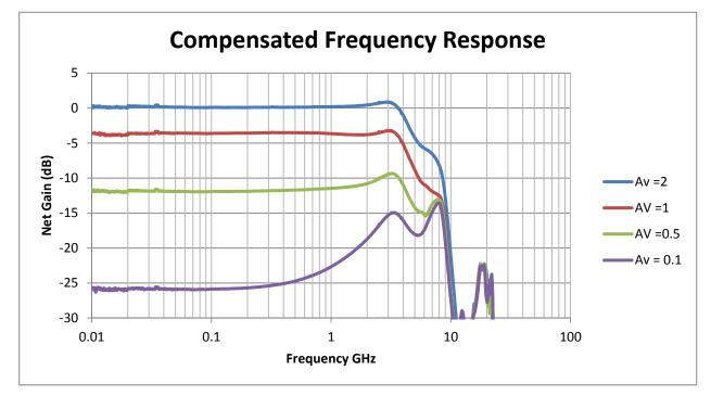
Figure 9 Measured frequency response for various gains
