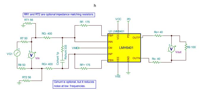
Figure 2 LMH5401 Basic Schematic (Note: Rf total = 200  $\Omega$ , there is 25  $\Omega$  on chip).
