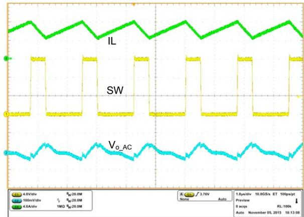
Figure 7.2 Switching Waveforms at  $V_{audio}=300mV$
