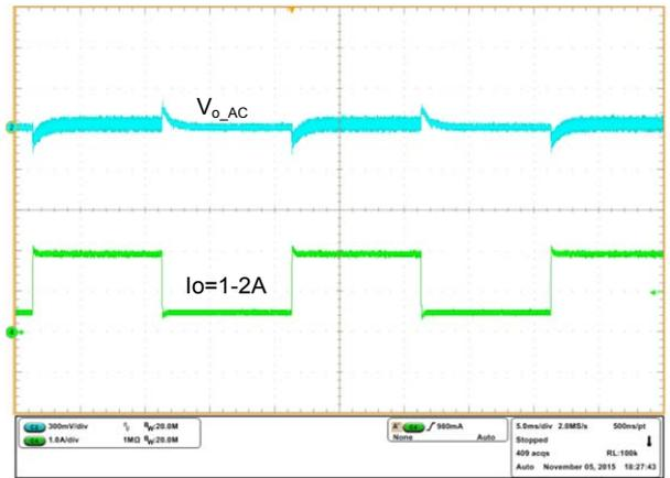
Figure 9.2 Load Transient ( $V_{\text{audio}}=300\text{mV}$ )
