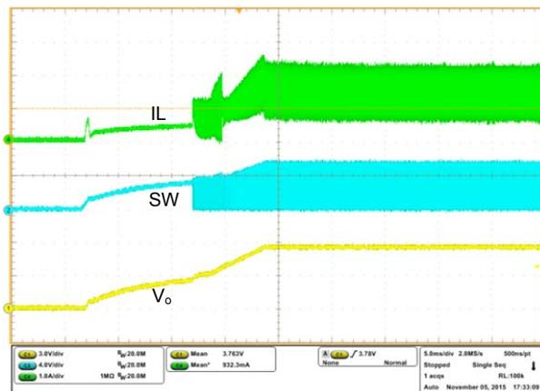
Figure 8.1 Startup Waveforms at  $V_{audio}=0V$
