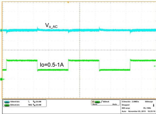
Figure 9.1 Load Transient ( $V_{\text{audio}}=0\text{V}$ )
