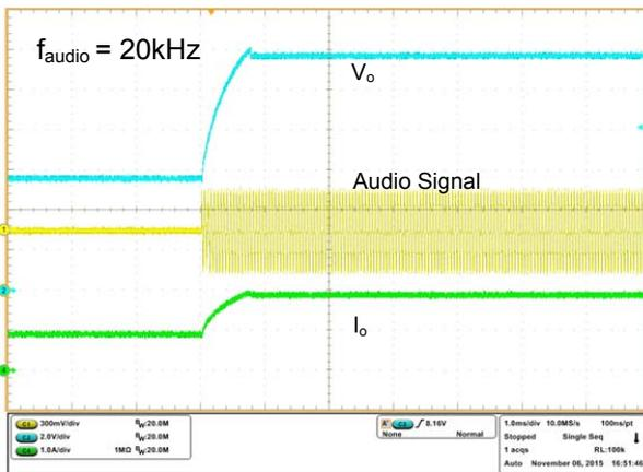
Figure 6.1 Output Voltage Transition at  $f_{audio}=20kHz$
