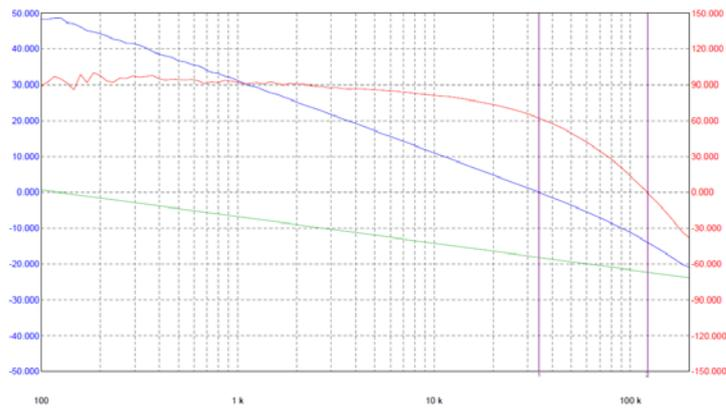
Figure 10.1 Loop Bode Plot ( $V_{\text{in}}=3.6\text{V}$ ,  $R_{\text{load}}=6\text{ ohm}$ )
