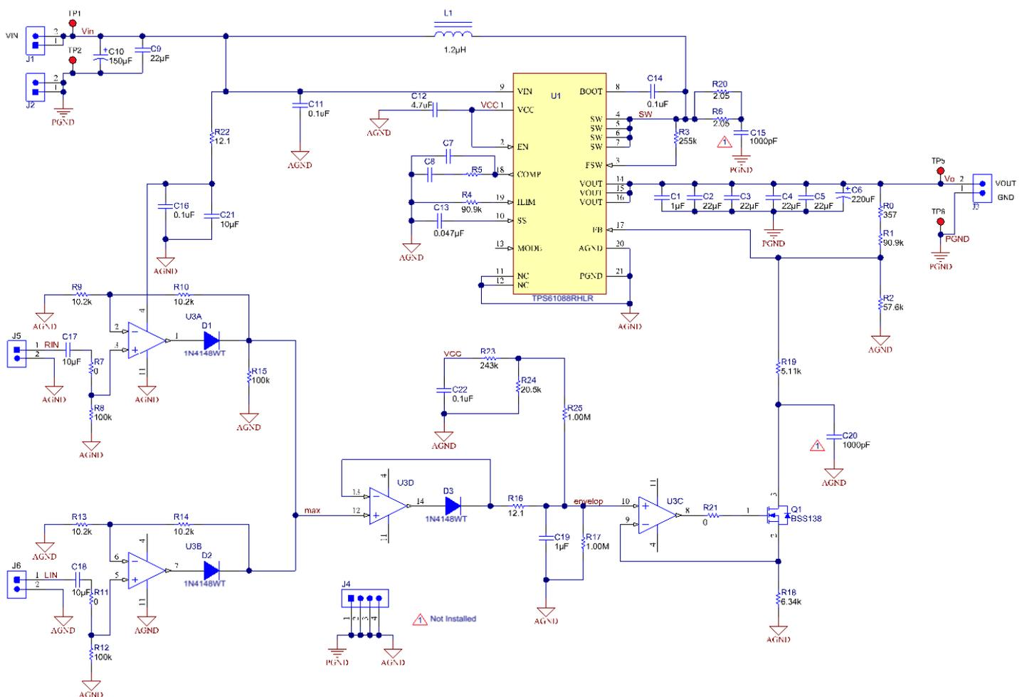
Figure 11. Schematic of the Reference Design with LMV324
