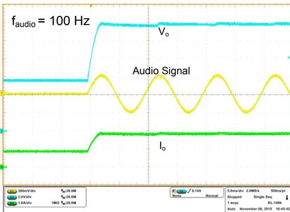
Figure 6.3 Output Voltage Transition at  $f_{audio}=100Hz$
