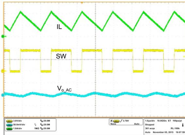
Figure 7.1 Switching Waveforms at  $V_{audio}=0V$
