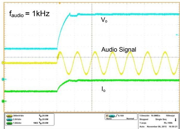
Figure 6.2 Output Voltage Transition at  $f_{audio}=1kHz$
