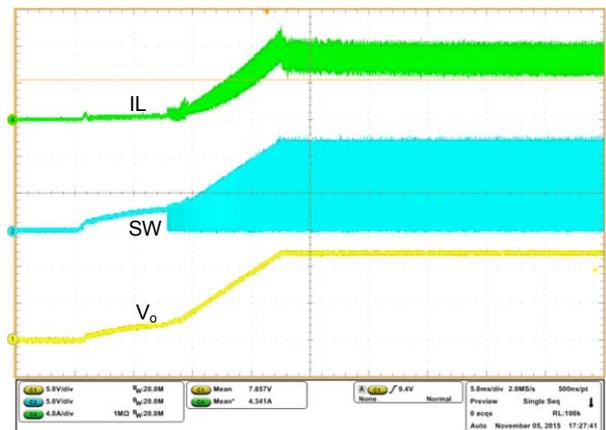
Figure 8.2 Startup Waveforms at  $V_{audio}=300mV$
