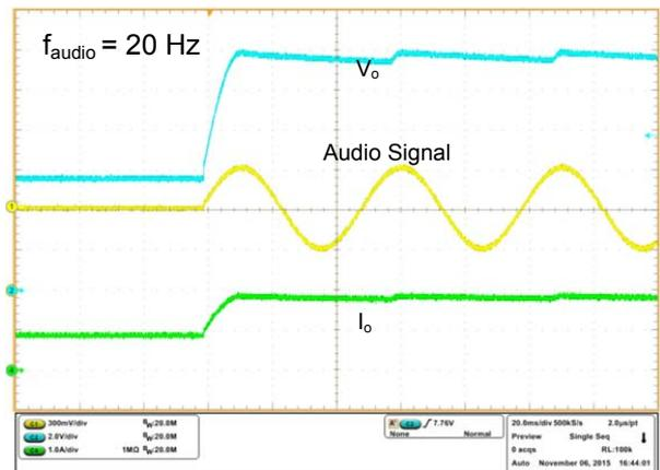
Figure 6.4 Output Voltage Transition at  $f_{audio}=20Hz$
