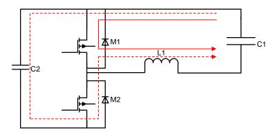
Figure 3. Power Stage When working as a Synchronous Boost Converter
