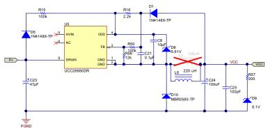
Figure 12. UC28880-Based Auxiliary Supply
