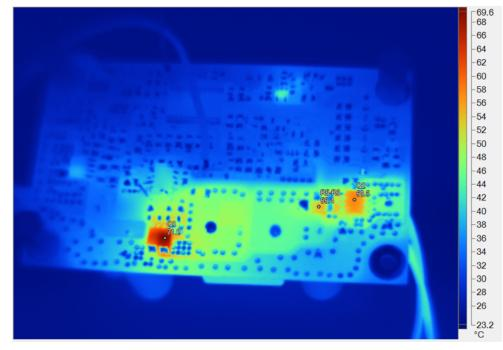
Figure 35. TIDA-00476 Thermal Image of Board—Bottom Side
