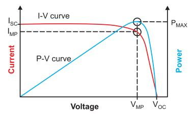
Figure 4. Solar Panel Characteristics I-V and P-V Curves
