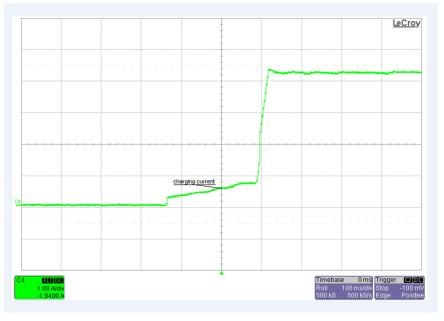
Figure 28. Ramp Up of Battery Charging Current and MPPT Action
