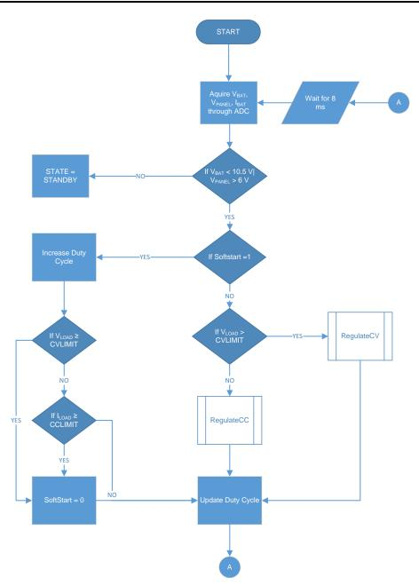
Figure 18. Flow Chart for CC-CV Driver State
