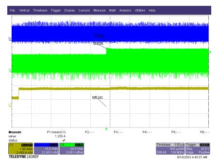
Figure 29. Change in Power Stage Operating Mode From Diode Emulation to Synchronous Buck
