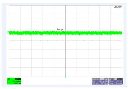
Figure 33. Current Ripple of CC-CV Driver Output Load When Operating in CC Region
