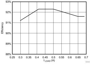
Figure 22. Efficiency Variation With DC Load Current Variation in CV Mode
