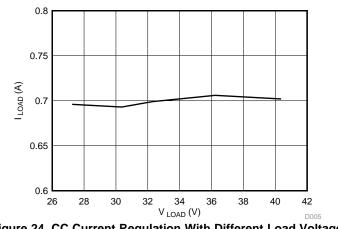
Figure 24. CC Current Regulation With Different Load Voltage
