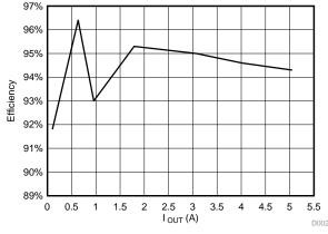
Figure 21. Efficiency Variation With Battery Charging Current
