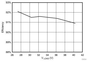
Figure 23. Efficiency Variation With DC Load Voltage Variation in CC Mode
