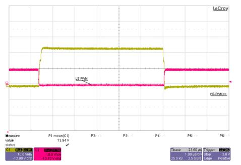
Figure 26 shows a zoomed-in image of the waveform with the complementary PWM outputs.
