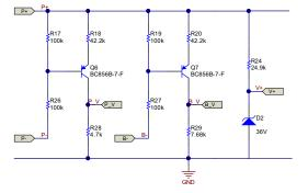
Figure 11. Battery and Panel Voltage Measurement Circuit
