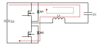
Figure 2. Power Stage When Working as Synchronous Buck Converter
