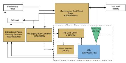
Figure 1. TIDA-00476 Block Diagram
