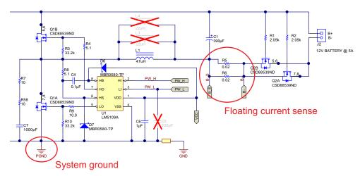
Figure 10. Floating Inputs for Battery Current Sensing
