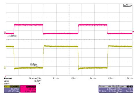
Figure 25. Complementary PWM Output from LM5109A Gate Driver
