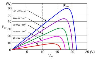
Figure 6. Solar Panel Output Power Variation Under Different Irradiation Conditions—Graph B [ 2]
