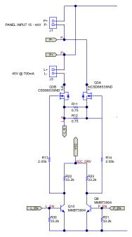
Figure 13. Bidirectional Power Directing Switches
