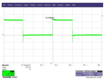
Figure 27. Switching Node Waveform When System is Working as Synchronous Buck Battery Charger
