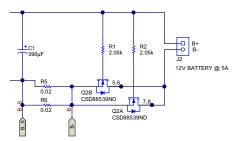
Figure 14. Battery Reverse Polarity Protection
