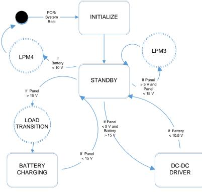
Figure 16. Firmware State Machine
