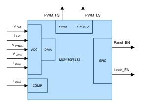
Figure 15. Block Diagram Showing MSP430 Interaction With System
