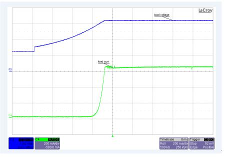
Figure 32. Ramp Up of CC-CV Driver Voltage and Current
