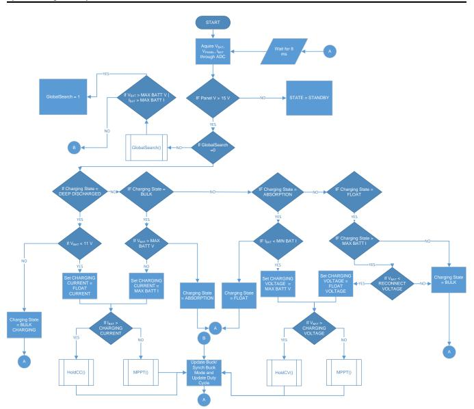
Figure 17. Flow Chart for Battery Charging State
