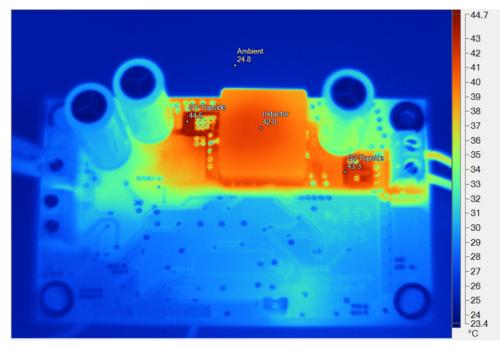
Figure 34. TIDA-00476 Thermal Image of Board—Top Side
