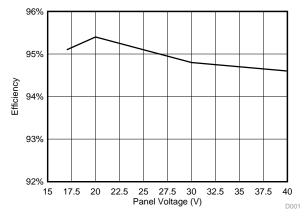
Figure 20. Variation of Solar Charger Efficiency With Panel Voltage at Maximum Battery Charging Current
