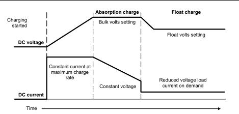
Figure 8. Lead Acid Battery Charging Stages
