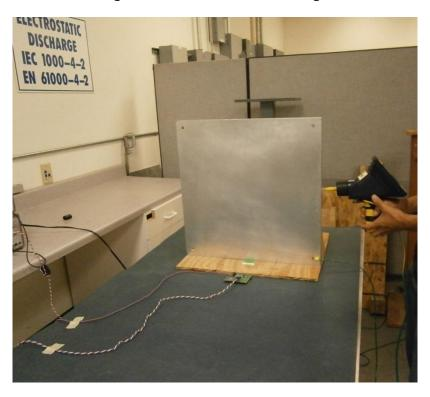
Figure B-2: 8kV ESD Vertical Contact Discharge
