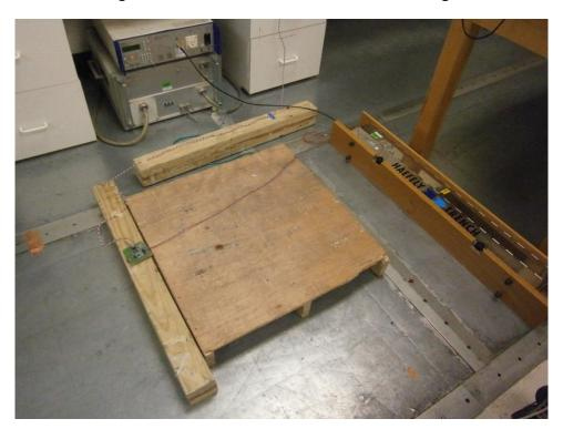
Figure B-4: EFT Test Setup
