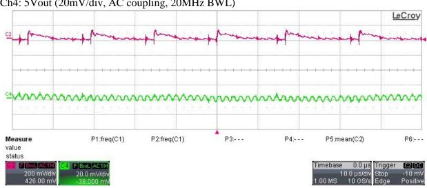
Ch2: 12Vout (200mV/div, 10us/div, AC coupling, 20MHz BWL) Ch4: 5Vout (20mV/div, AC coupling, 20MHz BWL)
