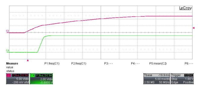
Ch2: 12Vout (5V/div, 5ms/div, 20MHz BWL) Ch4: 5Vout (2V/div., 20MHz BWL) Vin = 264Vac, 50Hz, full load on both outputs
