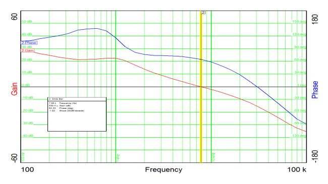
Current loop (TP23, TP24, TP25): Fco = 6.944KHz, PM = 68.22 deg, GM = 15.41dB.
