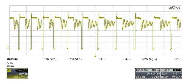
Ch1: TP3 switch node (100V/div, 2us/div, 200MHz BWL) Ch4: TP5 switch node (50V/div, 200MHz BWL) Vin = 230Vac, Vout = 27V, Iout = 6A
