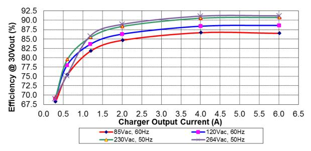
Efficiency of the converter (plug-to-plug) versus Vac & Output current with different Vout:
