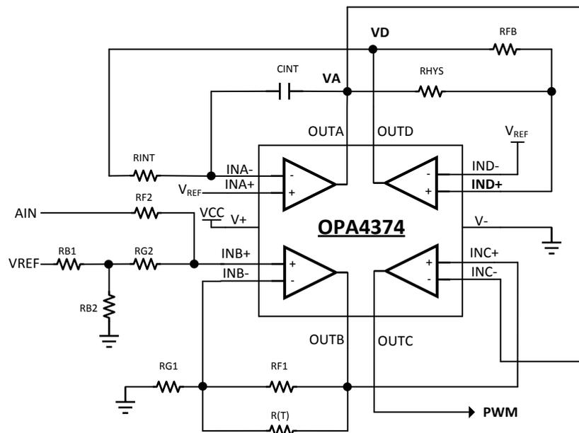
Figure 4. A2PWM Schematic
