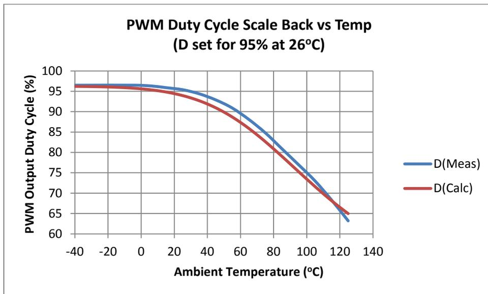
**Figure 8. PWM Duty Cycle Scale-Back vs Temp**
