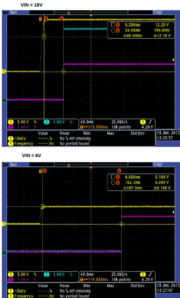
Figure 12.  $t_{\text{DELAY}}$  between VIN (Ch1) and VCC (Ch2), VREF (Ch3)
