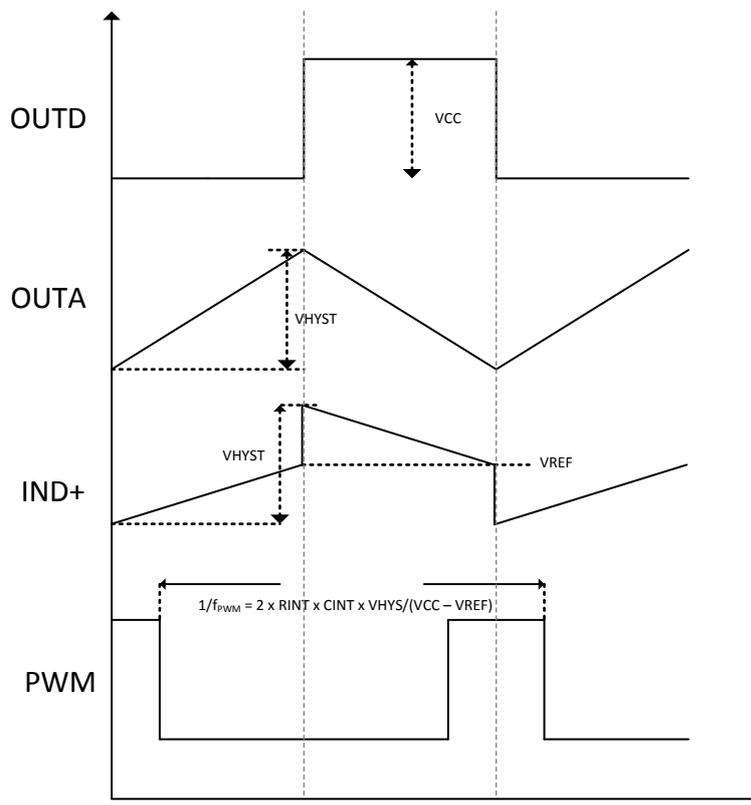
**Figure 5. A2PWM Voltage Waveforms**
