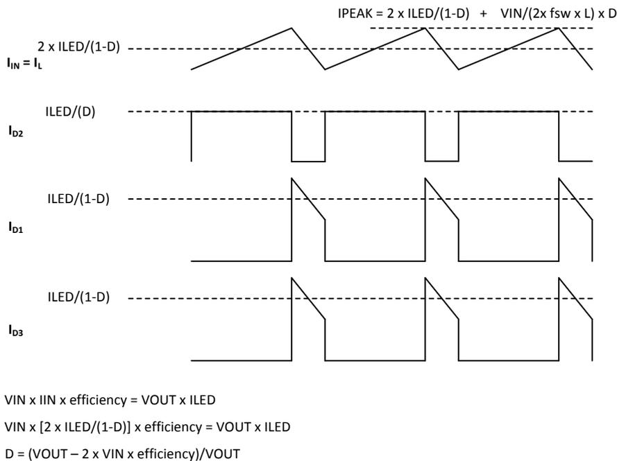
**Figure 3: Boost + Doubler Waveforms**
