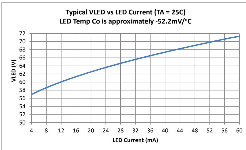
Figure 9. Typical VLED vs Current (SAW0LH0A from Seoul Semiconductor)
