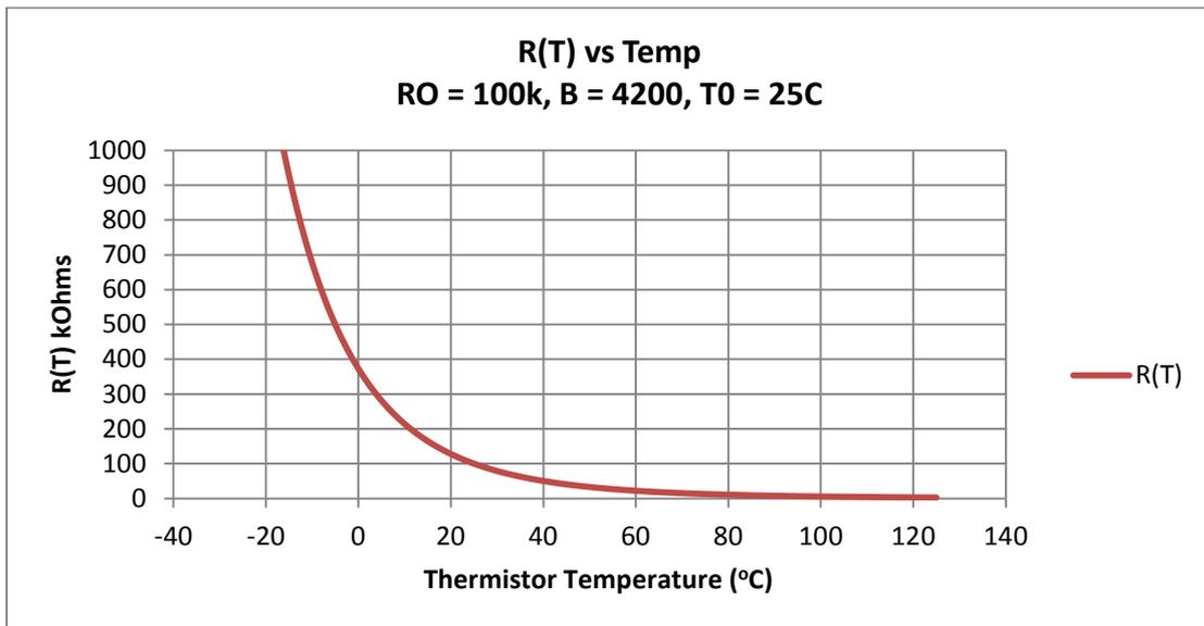
**Figure 6. NTC Thermistor Resistance vs Temperature**
