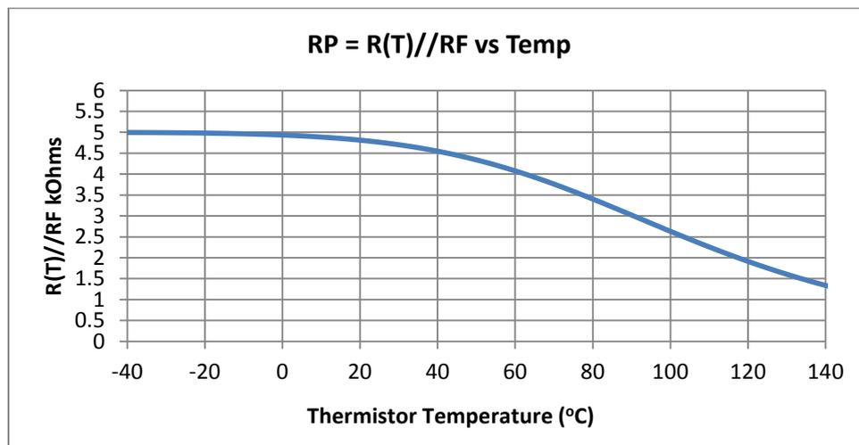
**Figure 7. Modified Thermistor Response**
