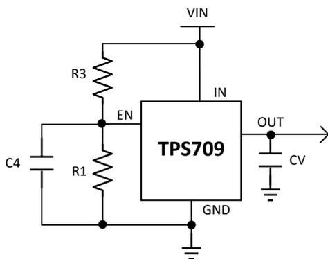
**Figure 11 VCC, VREF Generation Using the TPS709**
