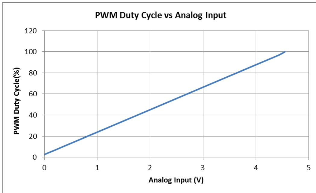
**Figure 10. PWM Duty Cycle vs AIN**
