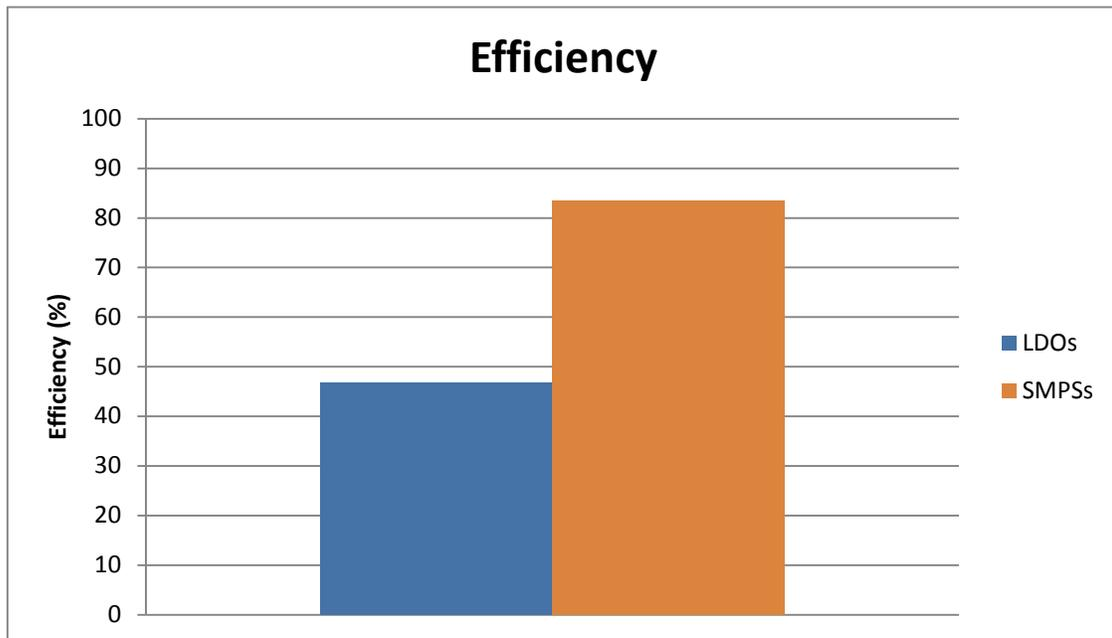
**Figure 5. Efficiency comparison of the LDO power solution to the SMPS power solution**
