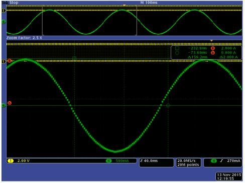
Figure 9. Motor #1 Peak 2A(RMS1.43A) at 1/32 micro-stepping
