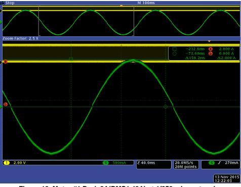
Figure 12. Motor #1 Peak 2A(RMS1.43A) at 1/256 micro-stepping
