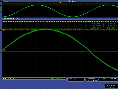
Figure 10. Motor #1 Peak 2A(RMS1.43A) at 1/64 micro-stepping
