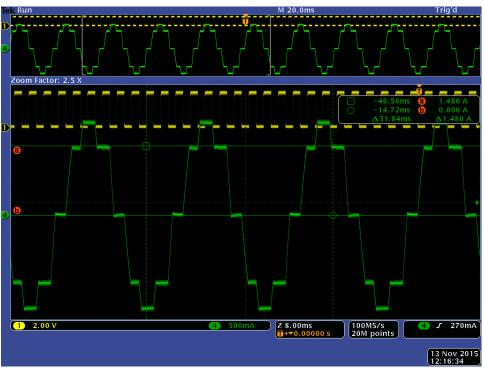
Figure 5. Motor #1 Peak 2A(RMS1.43A) at Half step
