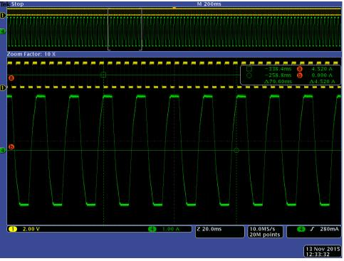
Figure 13. Motor #2 Peak 4.5A(RMS3.2A) at Full step
