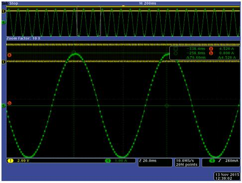
Figure 17. Motor #2 Peak 4.5A(RMS3.2A) at 1/16 micro-stepping
