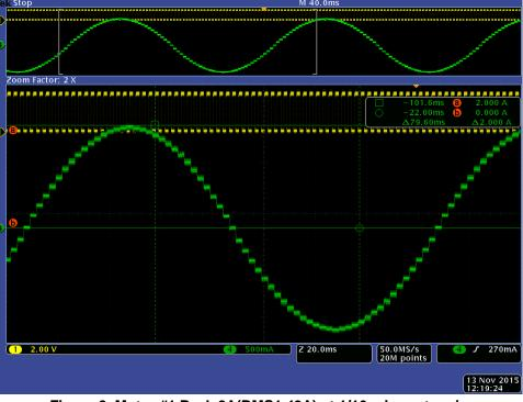
Figure 8. Motor #1 Peak 2A(RMS1.43A) at 1/16 micro-stepping
