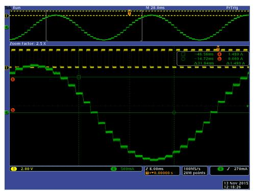
Figure 7. Motor #1 Peak 2A(RMS1.43A) at 1/8 micro-stepping
