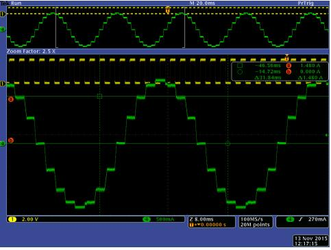
Figure 6. Motor #1 Peak 2A(RMS1.43A) at 1/4 micro-stepping
