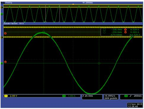
Figure 19. Motor #2 Peak 4.5A(RMS3.2A) at 1/64 micro-stepping
