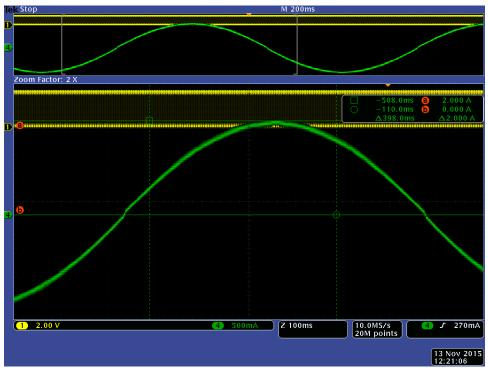
Figure 11. Motor #1 Peak 2A(RMS1.43A) at 1/128 micro-stepping
