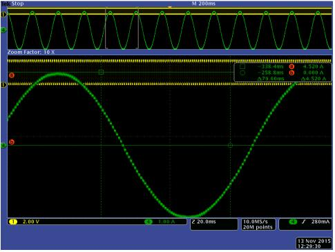
Figure 18. Motor #2 Peak 4.5A(RMS3.2A) at 1/32 micro-stepping
