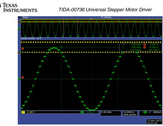
Figure 16. Motor #2 Peak 4.5A(RMS3.2A) at 1/8 micro-stepping
