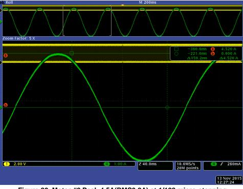
Figure 20. Motor #2 Peak 4.5A(RMS3.2A) at 1/128 micro-stepping
