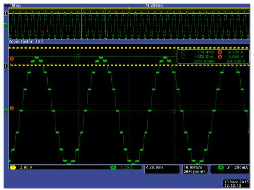
Figure 15. Motor #2 Peak 4.5A(RMS3.2A) at 1/4 micro-stepping
