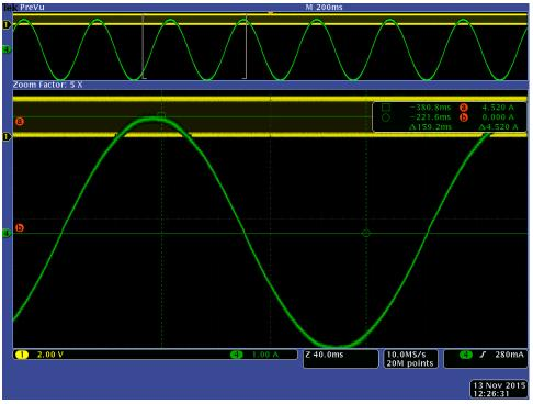
Figure 21. Motor #2 Peak 4.5A(RMS3.2A) at 1/256 micro-stepping
