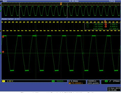
Figure 4. Motor #1 Peak 2A(RMS1.43A) at Full step
