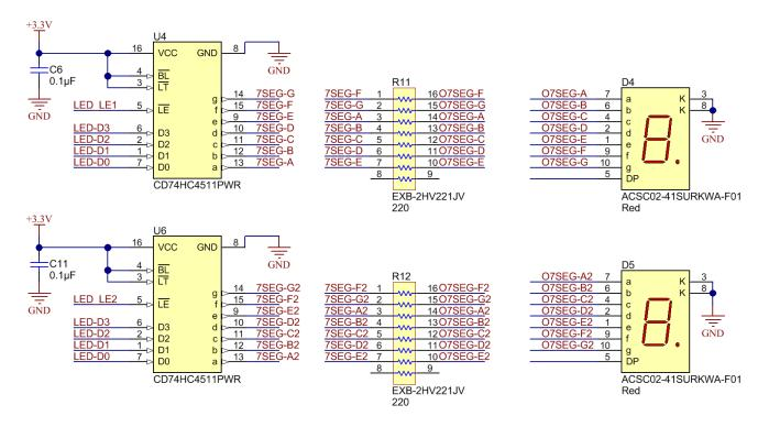
Figure 32: 7 Segment Displays and Drivers
