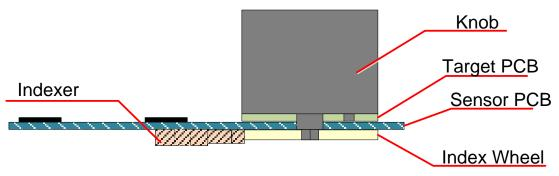
Figure 44: Mechanical Assembly
