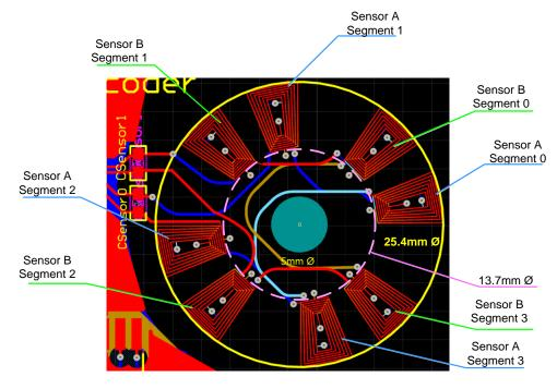
Figure 18: Multiple Sensor Segment Geometry
