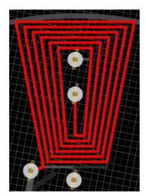
Figure 15: Trapezoidal Sensor configuration
