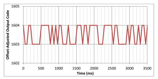
Figure 26: Sensor B Noise Level
