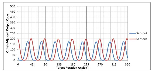
Figure 24: Output code variation due to target rotation at 1.0mm distance
