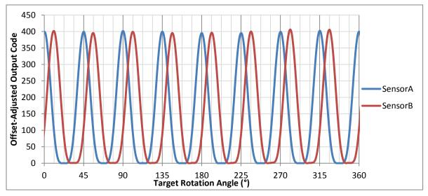
Figure 23: Output code variation due to target rotation at 0.5mm distance
