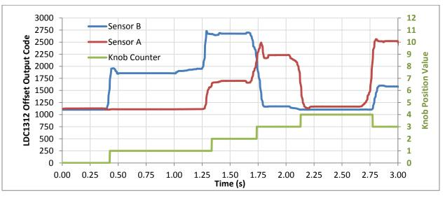
Figure 28: Example Sensor Data with Knob Position Value
