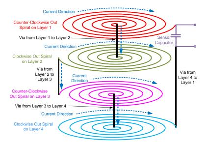
Figure 16: 4-Layer Inductor physical construction
