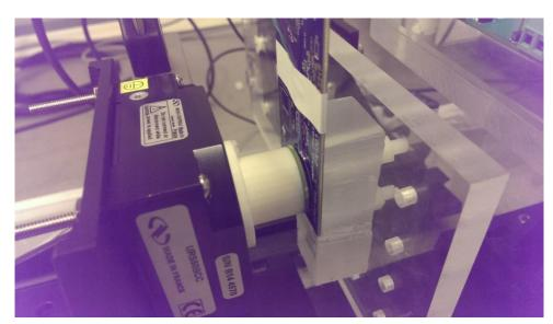
Figure 22: System used to measure rotational accuracy
