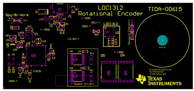
Figure 40: Sensor PCB Assembly Drawing
