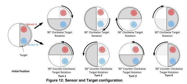
With the target initial position as shown in Figure 12, the target fully covers both sensors, and so the inductance of both sensors is at a minimum, as shown in Figure 13.
