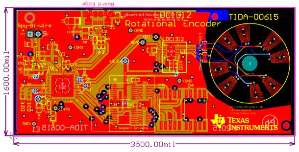
Figure 33: Multi-layer Sensor Print
