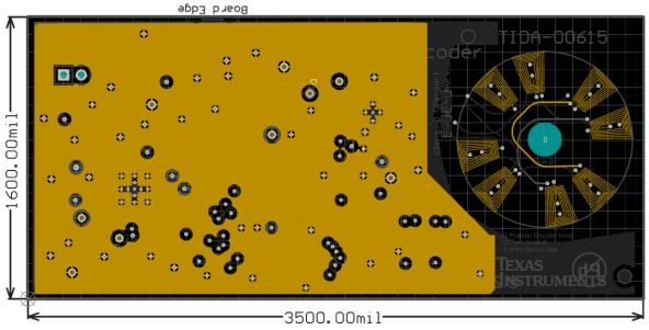
Figure 36: Sensor PCB Midlayer1 Routing
