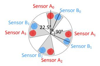
Figure 14: Equivalent Sensor placement for 16 position encoder
