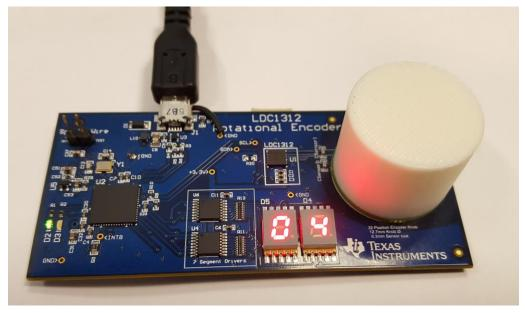
Figure 3: TIDA-00615 powered up by USB Connection after 4 steps
