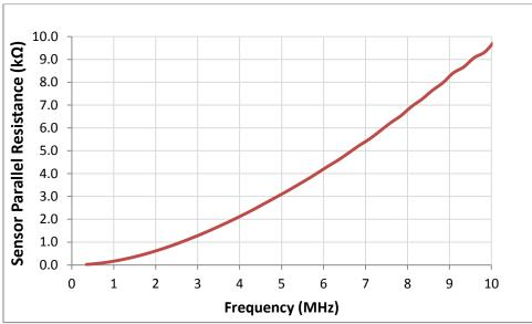
Figure 21: Parallel Resistance  $[\Omega]$  vs. Frequency sweep of each coil series
