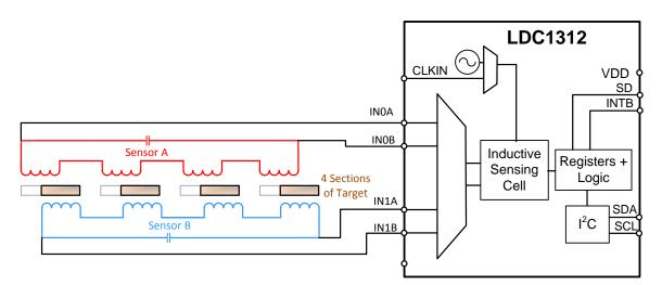
Figure 17: Multiple Section Sensor Connection
