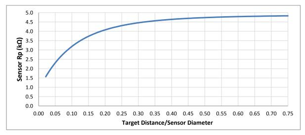
Figure 9: Sensor R<sub>P</sub> vs. Target Distance
