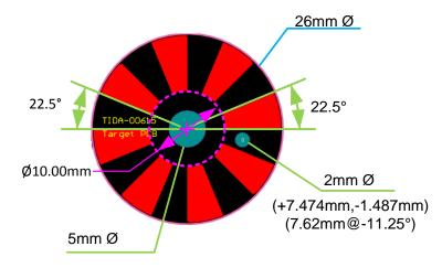
Figure 19: Target Dimensions
