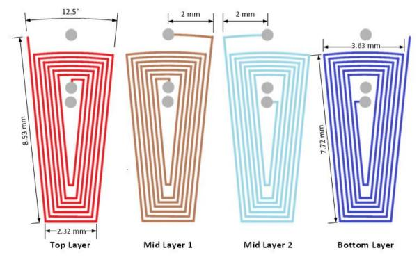
Figure 20: Trapezoidal Sensor Geometry and Layers
