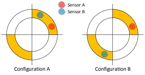
Figure 16: Equivalent configurations for sense inductors
