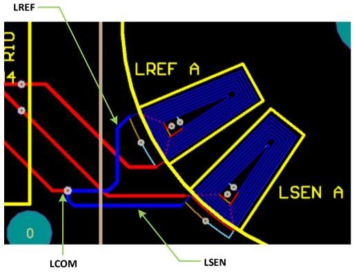
Figure 45: LSENSE, LREF and LCOM traces
