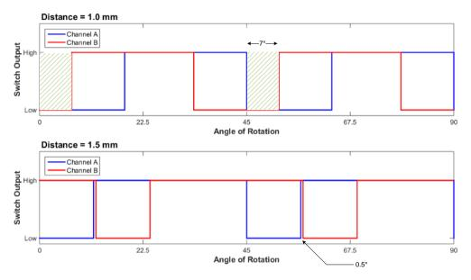
Figure 29: Channel trough overlaps
