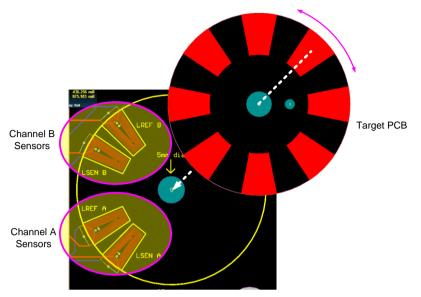
Figure 13: Sensor and Target configuration
