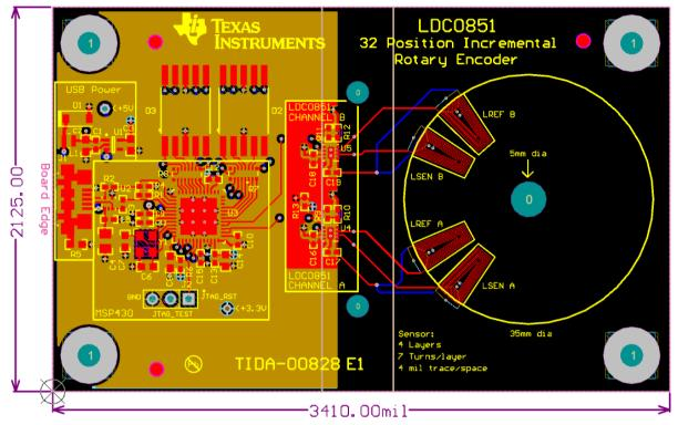
Figure 34: Sensor PCB Multi-layer
