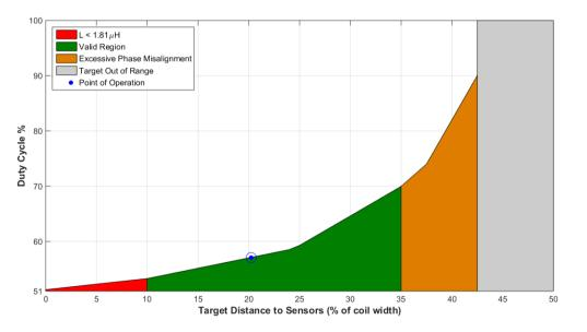
Figure 28: Target disk distance from sensors vs output duty cycles
