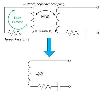
Figure 5: Electrical Model of Series Inductive Sensor
