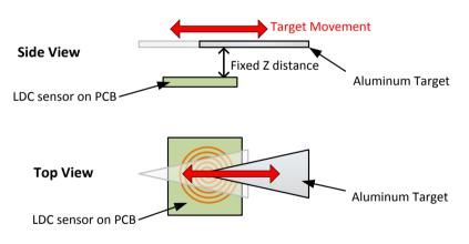
Figure 9: Lateral Position Sensing with LDC
