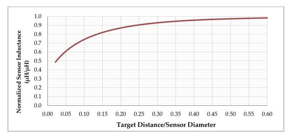
Figure 8: Normalized Sensor Response
