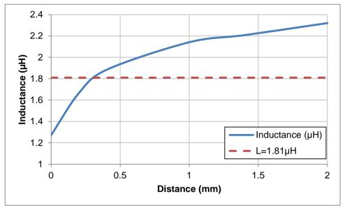
Figure 23: Sensor inductance vs target to sensor distance
