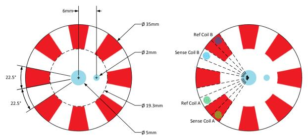
Figure 18: (Left) 32-Position target disk geometry, (Right) Sensor placement
