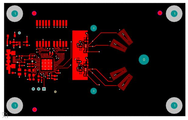
Figure 37: Sensor PCB Top Layer Routing
