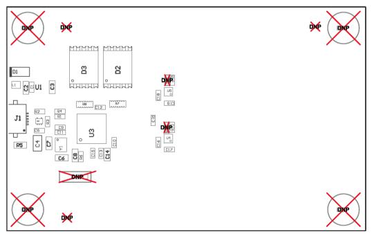
Figure 46: Sensor PCB Assembly Drawing
