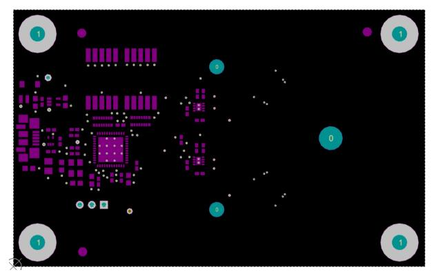
Figure 36: Sensor PCB Top Solder Mask
