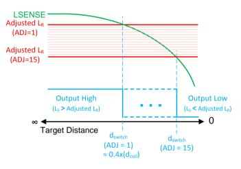
Figure 12: LDC0851 ADJ pin functionality
