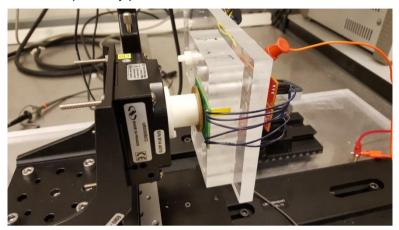
Figure 27: System used to measure rotational accuracy
