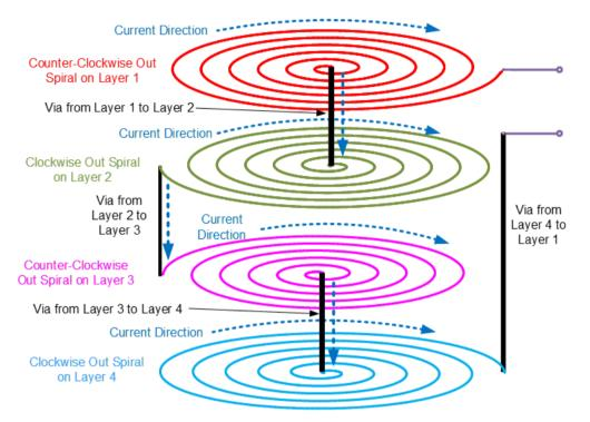
Figure 22: 4-Layer Inductor/sensor physical construction
