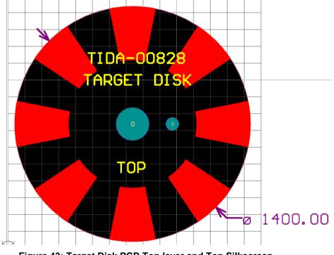
Figure 43: Target Disk PCB Top layer and Top Silkscreen
