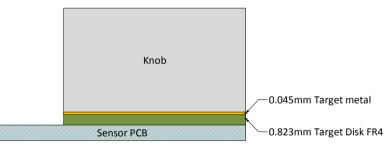
Figure 24: Target Disk – Sensor spacing using target disk PCB
