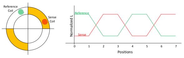
Figure 17: Reference coil placement and inductance shifts
