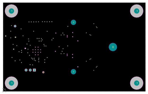
Figure 41: Sensor PCB Bottom Solder Mask
