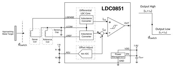
Figure 10: LDC0851 Block Diagram
