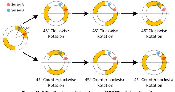
Figure 15: 8-Position target disk and sensor (SENSE coils) configuration
