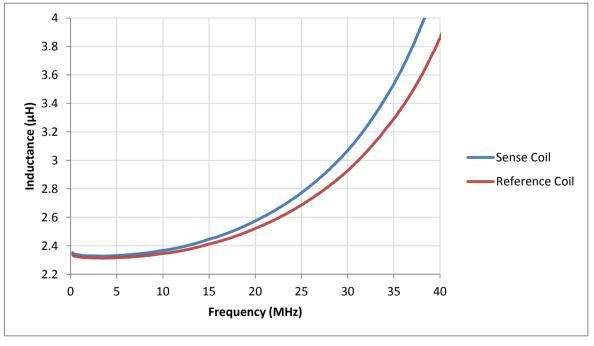
Figure 26: Coil characteristics using impedance analyzer
