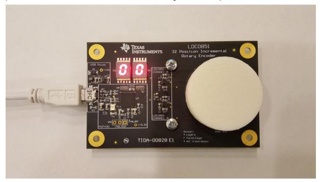
Figure 3: TIDA-00828 powered up by USB Connection
