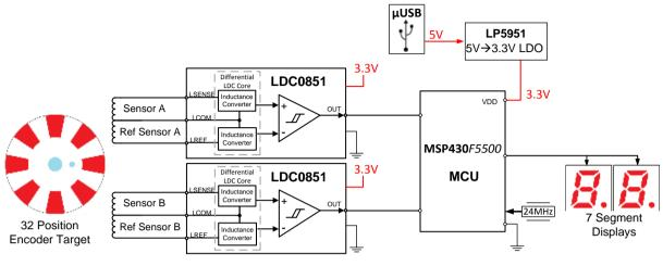
Figure 2: TIDA-00828 System Block Diagram
