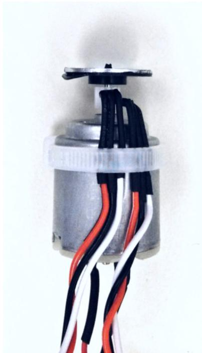
**Figure 3. Encoder Setup**
