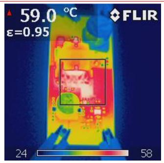
IR thermal image taken at steady state at 400 mA load and VIN = 16 V for two minutes with no airflow (4 Layer board, 1 Oz copper layer)
