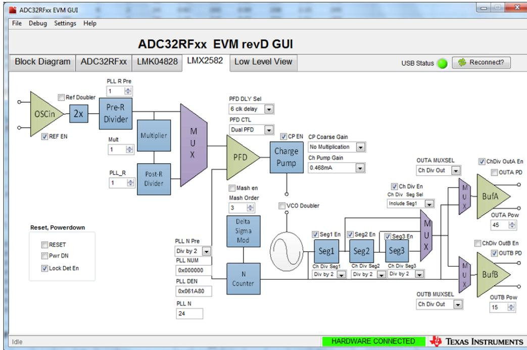
Figure 2. LMX2582 Programming Tab
