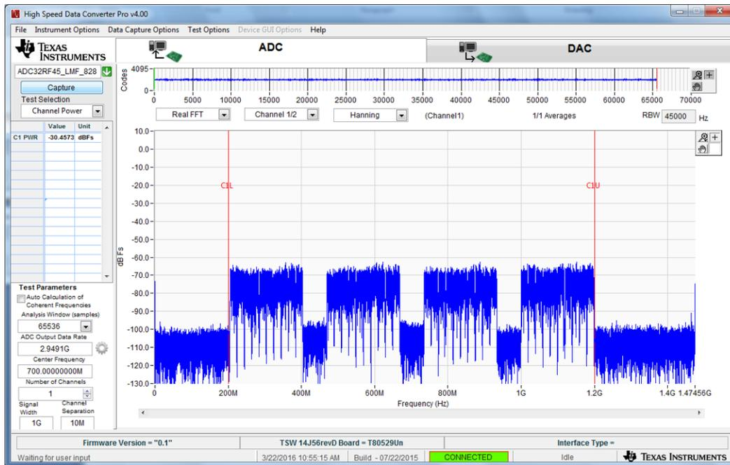
Figure 5. ADC32RF45 Capture With 1-GHz Signal Bandwidth
