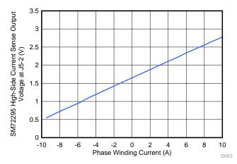
Figure 37. SM72295 Current Sense Amplifier Output Voltage at J5-2 Sampled at PWM Center versus Measured Phase Winding Current (Fluke Ampere Meter)
