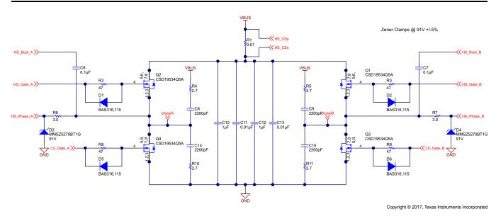
Figure 6. Schematic of Full-Bridge Power Stage
