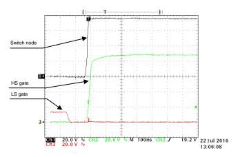
Figure 26. Phase A Rising Switch Node Voltage, High-Side, and Low-Side Gate to GND at 1-A Output Current
