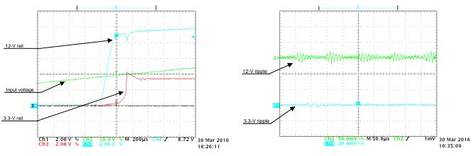
Figure 19. Point-of-Load Power-Up at 50-V DC Input
