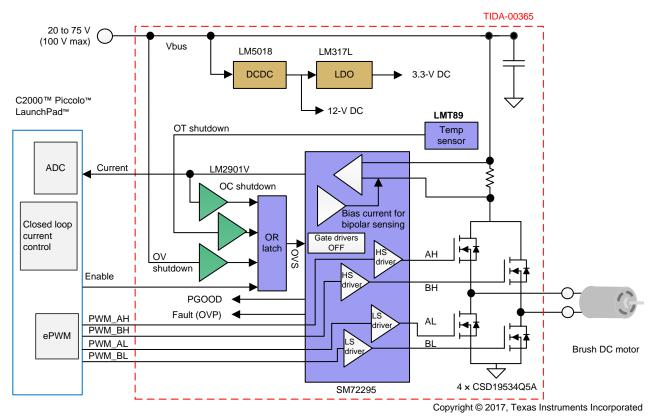
Figure 2. TIDA-00365 Block Diagram
