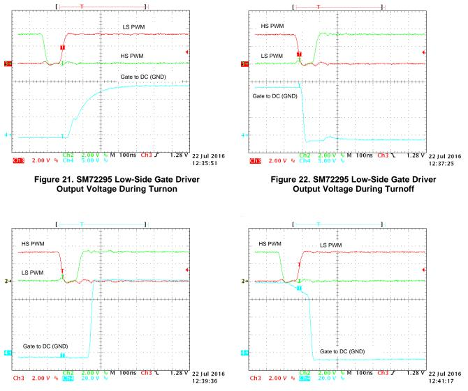
Figure 23. SM72295 High-Side Gate Driver **Output Voltage versus GND During Turnon**
