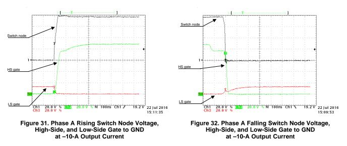
The figures in this section show that the full-bridge switching exhibits hard-switching of MOSFETs as well as soft switching depending on the output current. Also, the Miller capacity impact on the gate to source voltage can be seen: a faster transition with higher currents.
