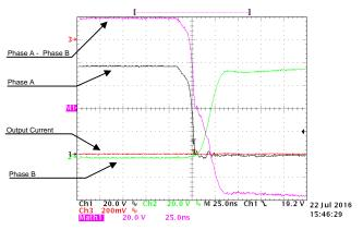
Figure 36. Falling Edge of Output Voltage, Phase A and B Voltage to GND at -10-A Output Current
