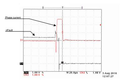
Figure 51. Short-Circuit Current Between Motor Terminals Phase A to Phase B and SM72295 nFAULT Signal
