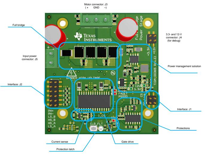
Figure 15. TIDA-00365 Functional Blocks (Top View)
