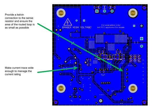
Figure 57. Bottom Layer (Flip View)
