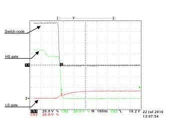
Figure 28. Phase A Falling Switch Node Voltage, High-Side, and Low-Side Gate to GND at -1-A Output Current
