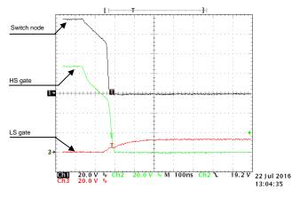
Figure 25. Phase A Falling Switch Node Voltage, High-Side, and Low-Side Gate to GND at 1-A Output Current
