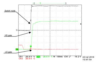
Figure 29. Phase A Falling Switch Node Voltage, High-Side, and Low-Side Gate to GND at 10-A Output Current
