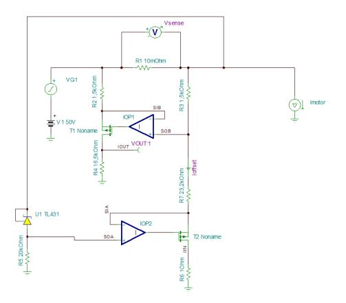
Figure 11. TI-TINA™ Simulation Circuit of Implement Current Sense Solution
