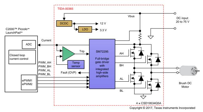
Figure 1. TIDA-00365 Simplified Block Diagram and C2000 MCU for Brushed DC Drive Current Control
