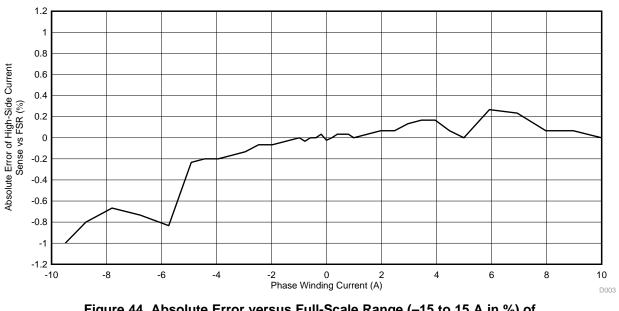
Figure 44. Absolute Error versus Full-Scale Range (–15 to 15 A in %) of SM72295 Current Sense Amplifier Output
