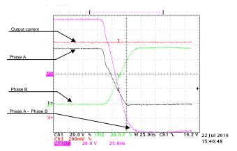
Figure 34. Falling Edge of Output Voltage, Phase A and B Voltage to GND at 10-A Output Current
