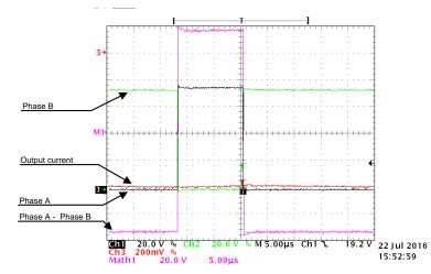
Figure 37. Output Voltage, Phase A and B Voltage to GND at -10-A Output Current Over One PWM Cycle
