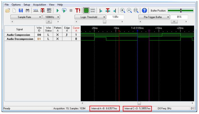
Figure 39. CPU Usage for Audio Codec
