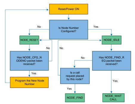
Figure 10. Control-State Machine One
