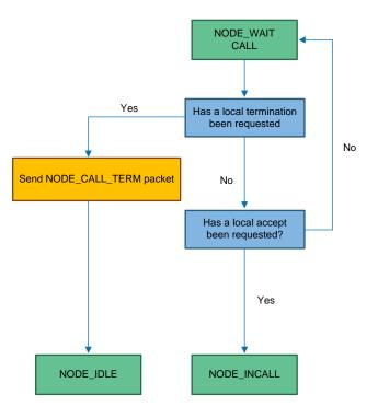
Figure 12. Control-State Machine Three
