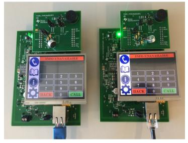
Figure 28. First Power Up of the Design
