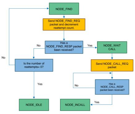
Figure 11. Control-State Machine Two
