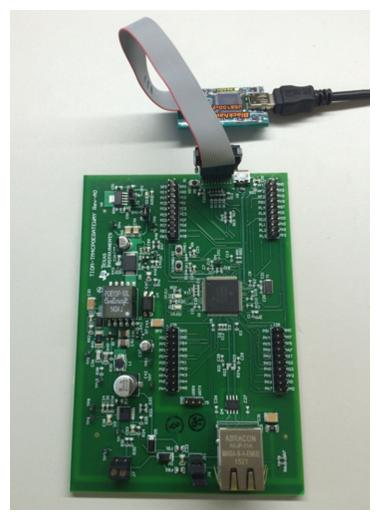
Figure 17. Connecting the Debugger
