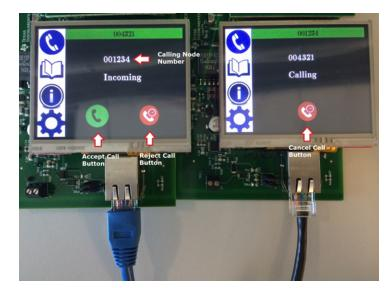
Figure 36. Display Status When Placing a Call
