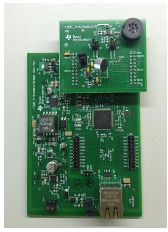
Figure 15. Mounting Audio Board
