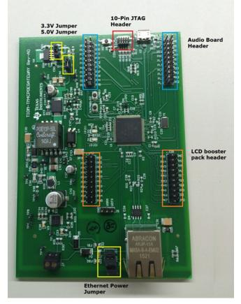
Figure 14. TIDM-TM4C129POE Connector and Shunt Layout
