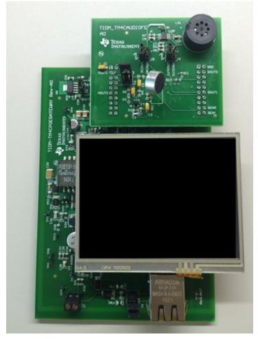
Figure 16. Mounting the LCD Touch Panel
