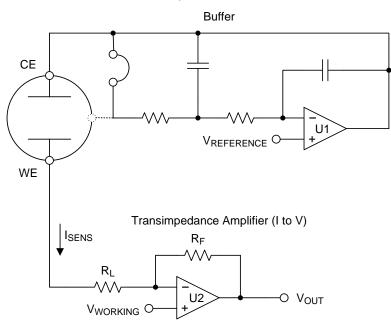
Figure 4. Modified Circuit for Two-Terminal Sensors
