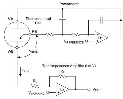
Figure 3. Simplified Electrochemical Measurement Circuit
