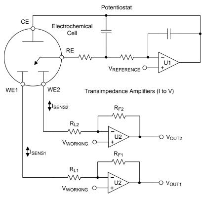
Figure 5. Four-Terminal Sensor Circuit
