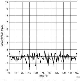
Figure 10. Sensor Baseline in Open Room Air
