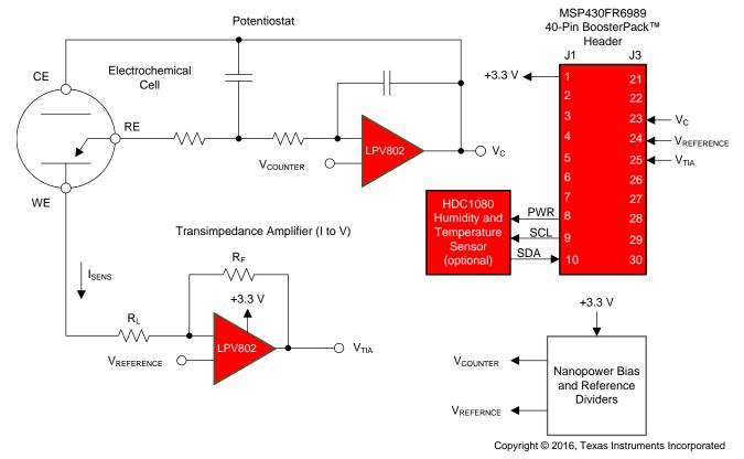
Figure 1. TIDA-00854 Block Diagram
