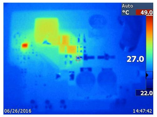
Figure 19. Thermal Image of Boost-to-Battery
