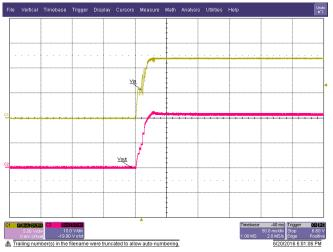
Figure 13. Startup Into No Load (Current Sense Comparator Reference Voltage Set to 0 V) at 12  $V_{\mbox{\tiny IN}}$
