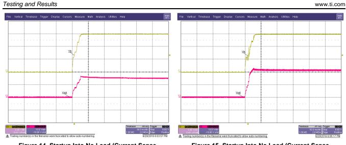
Figure 14. Startup Into No Load (Current Sense Comparator Reference Voltage Set to 2.5 V) at 15  $V_{IN}$
