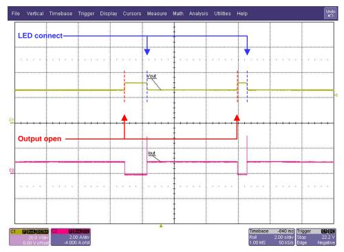
Figure 31. Boost-to-Battery Open Circuit Protection
