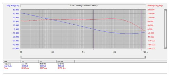
Figure 33. 12-V<sub>IN</sub> Loop Response Showing a Stable System With Gain Margin: 8.9 dB and Phase Margin: 99.7°
