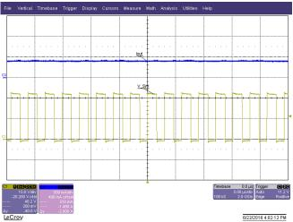
Figure 21. 12-V<sub>IN</sub> and 0-V Reference on Current Sense **Comparator Provides Maximum Output Current**
