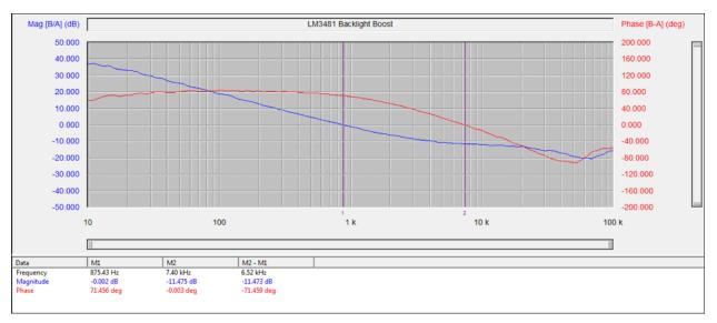
Figure 18. 12-V<sub>IN</sub> Loop Response Showing a Stable System With Gain Margin: 11.4 dB and Phase Margin: 71.4°
