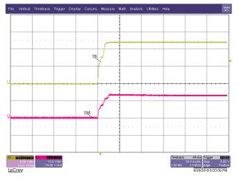
Figure 12. Startup Into No Load (Current Sense Comparator Reference Voltage Set to 2.5 V) at 12  $V_{\mbox{\tiny IN}}$
