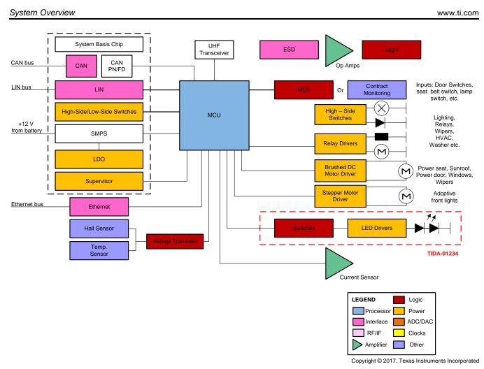
Figure 2. Automotive LED Lighting Example Highlighting TIDA-01234
