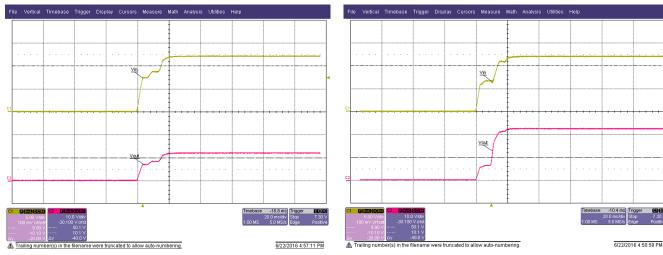
Figure 26. Startup Into No Load (Current Sense Comparator Reference Voltage Set to 2.5 V) at 12  $\rm V_{IN}$
