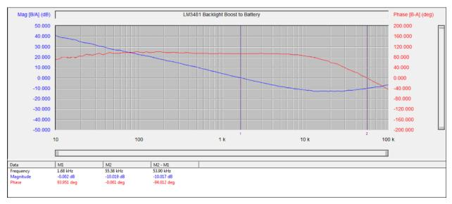
Figure 32. 6-V<sub>IN</sub> Loop Response Showing a Stable System With Gain Margin: 10.0 dB and Phase Margin: 93.95°
