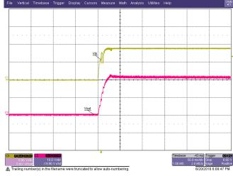
Figure 10. Startup Into No Load (Current Sense Comparator Reference Voltage Set to 2.5 V) at 9 V\_{ $\mbox{\tiny IN}}$
