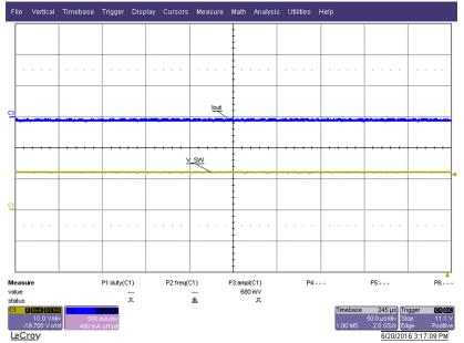
Figure 9. 12 V<sub>IN</sub> and 2.5-V Reference on Current Sense Comparator Provides Maximum Output Current
