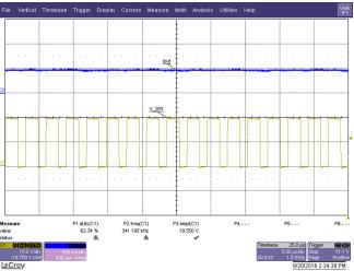
Figure 7. 12-V<sub>IN</sub> and 0-V Reference on Current Sense **Comparator Provides Maximum Output Current**
