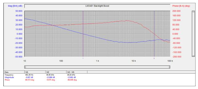
Figure 17. 6-V<sub>IN</sub> Loop Response Showing a Stable System With Gain Margin: 13.8 dB and Phase Margin: 86.5°
