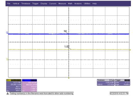
Figure 23. 12-V<sub>IN</sub> and 2.5-V Reference on Current Sense Comparator Provides Maximum Output Current
