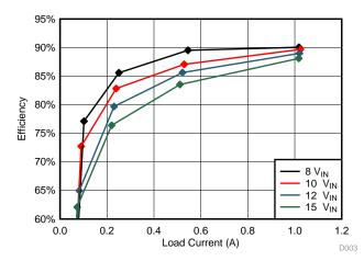
Figure 20. Boost-to-Battery Efficiency versus Load Current at Various Input Voltages
