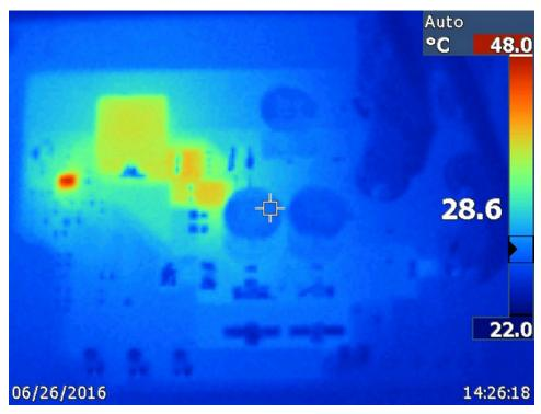
Figure 5. Thermal Image of Boost Configuration
