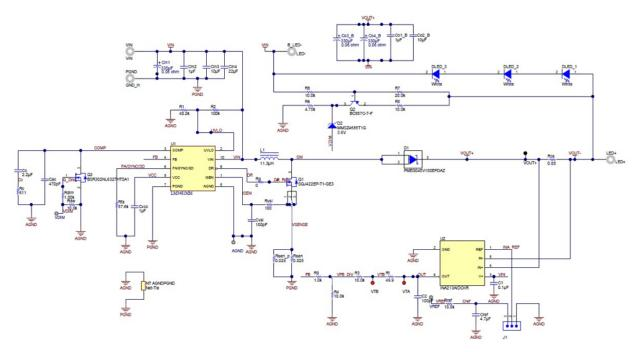
Figure 4. Boost-to-Battery Configuration and LM3481 Schematic
