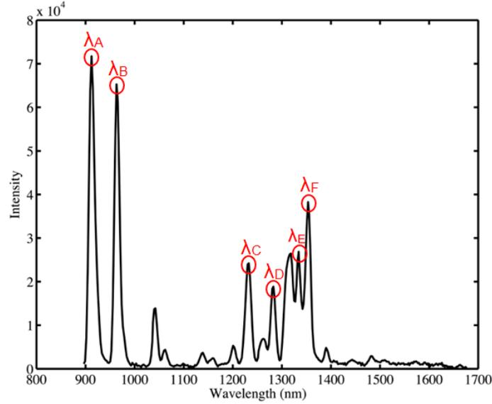
**Figure 1: The spectrum of the argon test source**
