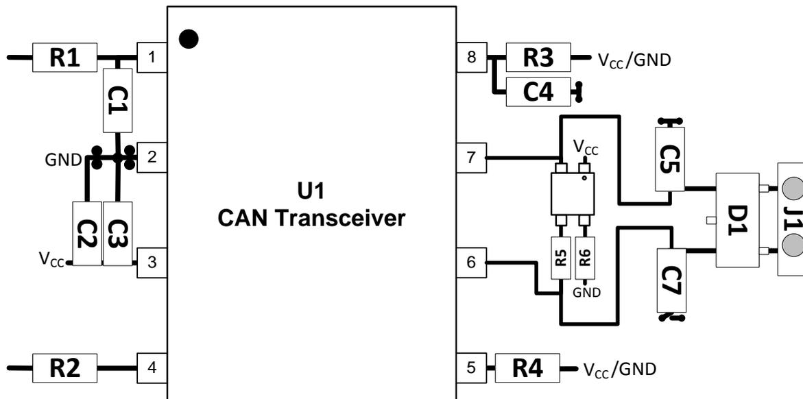
Figure 14: CAN Selectable Termination TLP175A Layout Example
