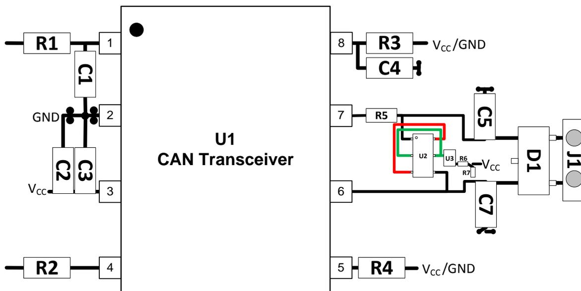
Figure 15: CAN Selectable Termination CSD87502Q2 and CSD17483F4 Layout Example
