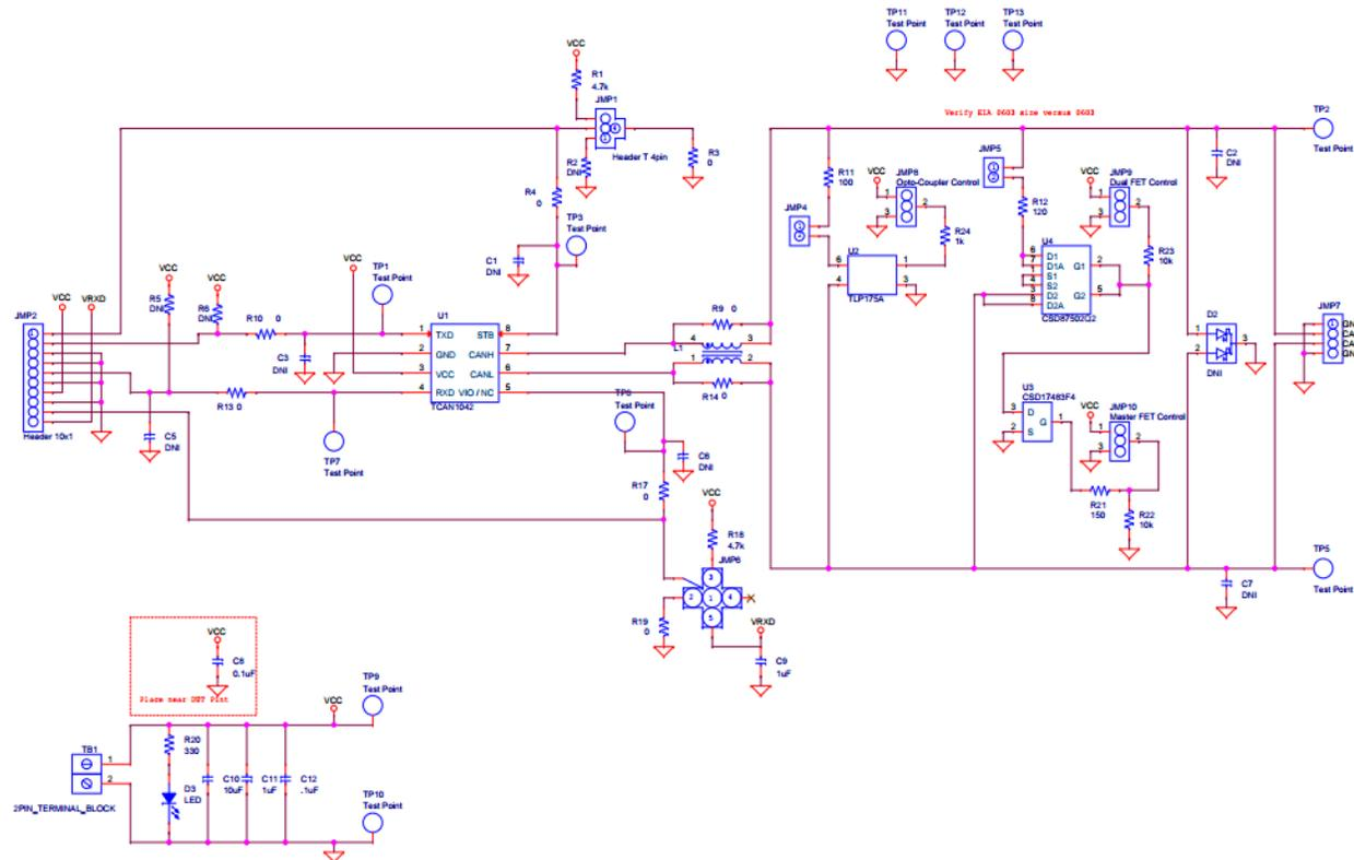
Figure 13: CAN Selectable Termination Evaluation Board Schematic
