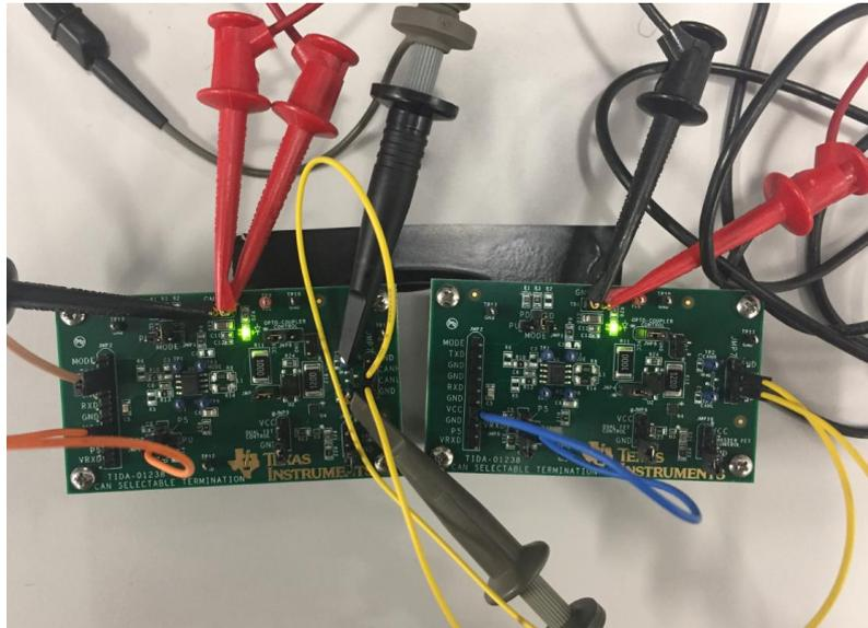
Figure 3: CAN Selectable Termination Evaluation Module Photorelay Solution Setup
