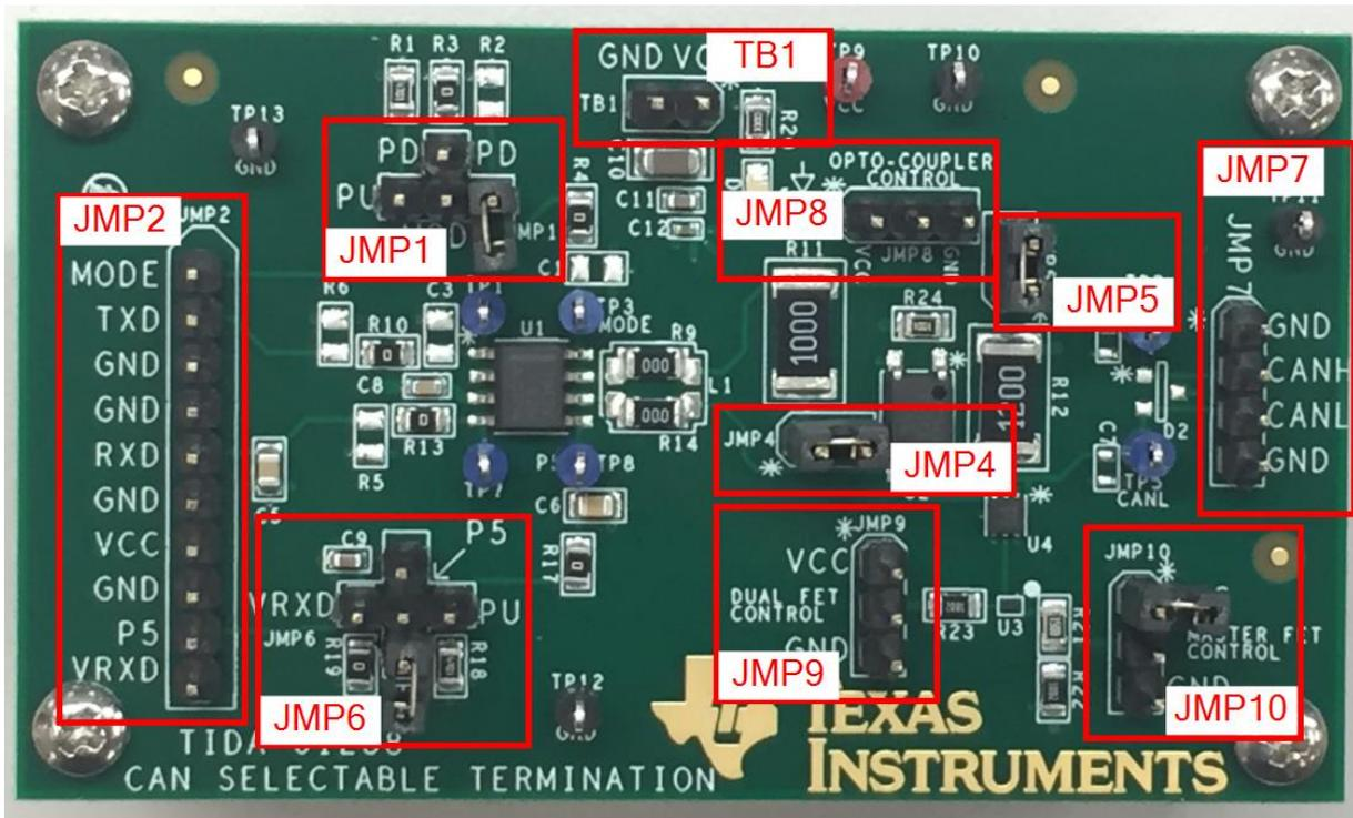
Figure 1: CAN Selectable Termination Evaluation Board
