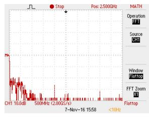
Figure 24. Class D Differential FFT Output
