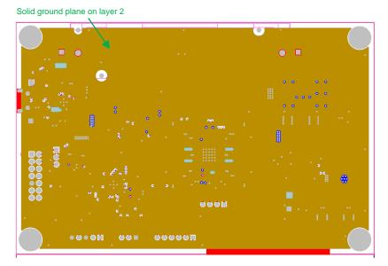
Figure 29. PCB Inner Layer 2 (Ground Plane Layer) Layout
