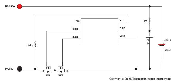
Figure 4. bq29705 Typical Application Diagram
