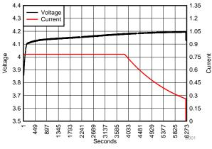
Figure 25. Charge Cycle Plot
