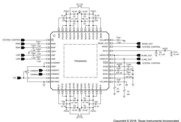
Figure 8. TPA3004D2 Typical Application Diagram
