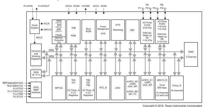
Figure 6. MSP430FR5735 Typical Block Diagram
