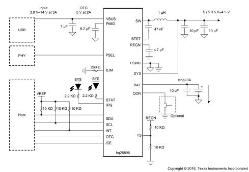
Figure 2. bq25896 Typical Application Diagram
