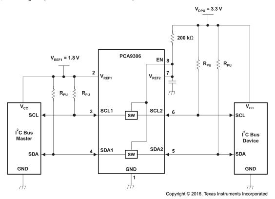
Figure 10. PCA9306 Typical Application Diagram
