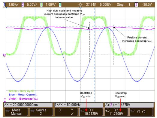
Figure 28. Bootstrap V<sub>DD</sub> Ripple at 16 kHz
