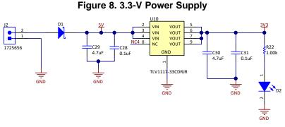
Table 4 shows the power consumption by the different circuit biased by the 3.3-V rail. There are six digital isolators ISO7721, an indication LED, and GaN fault combination circuitry using AND gates powered from this 3.3-V rail. The current consumption is considered maximum worst case from their respective data sheets. The 2.4 mA for ISO7721 device is the current consumed on the low-voltage side bias at 3.3 V and for a square waveform with a 1-Mbps transmission rate.
