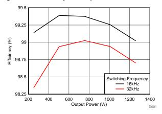
Figure 18. Efficiency vs Output Power - no Airflow
