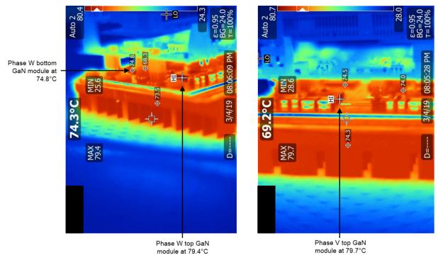
Figure 20. Thermal Data at 3.5 A, 16 kHz
