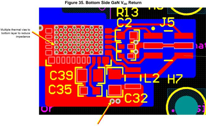
Vias to free V<sub>DD</sub> currents return through J5 connector to HVBUS\_RTN instead of through switching current plane – needed to reduce noise on V<sub>DD</sub> and prevent false UVLO
