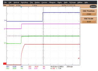
Figure 89. Start-Up Behavior of All Bias Power Supplies—Start Initiated by EN12 From 12-V Battery Terminal: (Blue = P12V, Violet = P3V3, Green = P10V, and Red = VIN\_LM)
