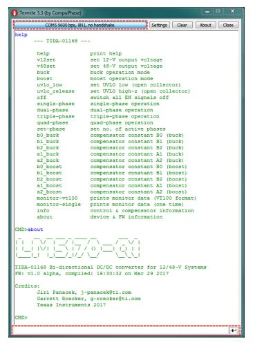
Figure 61. Interfacing TIDA-01168 With Serial Terminal Using Termite 3.3
