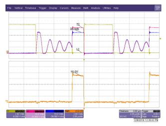
Figure 68. Switching Waveforms With Fixed Dead-Time Settings (R906 = 10 k)
