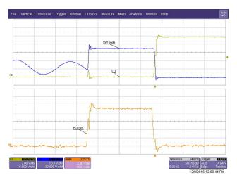
Figure 67. Switching Waveforms With Adaptive Dead-Time Settings (Detail)
