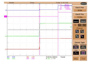
Figure 81. External Watchdog Behavior During Start-Up: (Blue = nRST, Violet = NSHDN, Green = P10V, and Red = P3V#)
