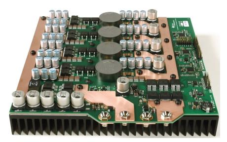
Figure 12. TIDA-01168 Assembled Prototype
