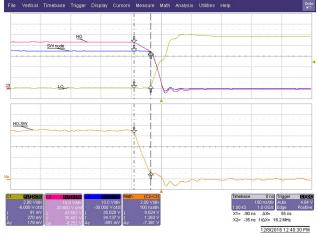
Figure 69. Switching Waveforms With Fixed Dead-Time Settings (R906 = 10 k) - Detail
