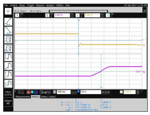
Figure 7. Propagation Delay (High to Low)
