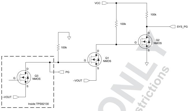
Figure 1-7. PG Pin Level Shifter
