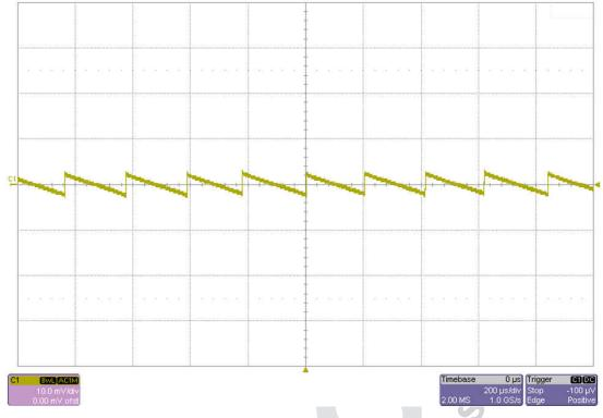
Figure 3-13. Output Voltage Ripple (5 V<sub>IN</sub>, 1-mA Load)
