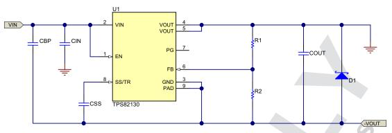
Figure 1-8. Installation of Schottky Diode D1 Required, if Installing CBP
