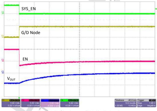
Figure 3-18. Shutdown on EN (5 V<sub>IN</sub>, No Load)
