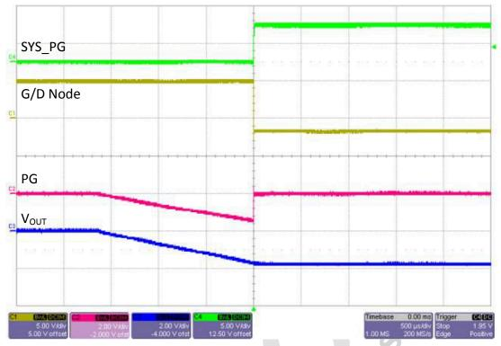
Figure 3-19. PG on Start-up (5 V<sub>IN</sub>, No Load)
