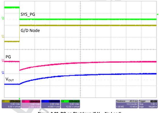
Figure 3-20. PG on Shutdown (5 V<sub>IN</sub>, No Load)
