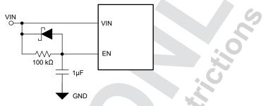
Figure 1-5. EN Pin Delay Using an RC Filter and Schottky Diode
