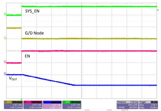
Figure 3-17. Start-up on EN (5 V<sub>IN</sub>, No Load)
